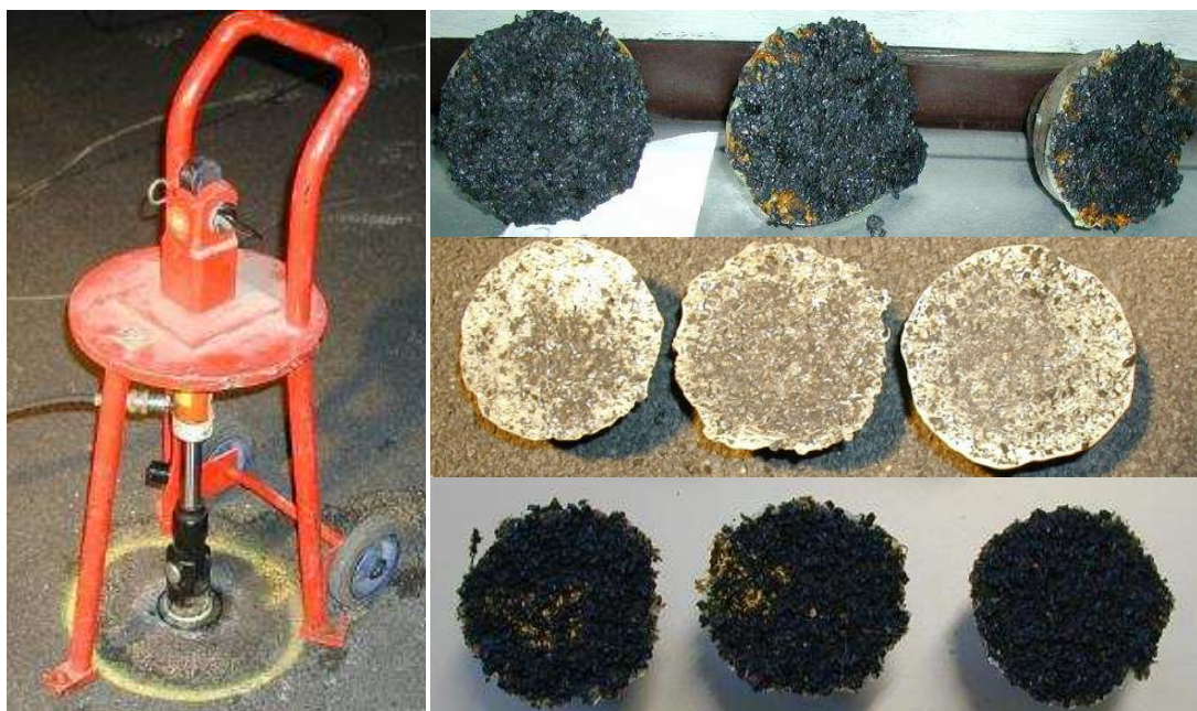
Figure 3 Setup for bonding tests and kinds of surface coating
