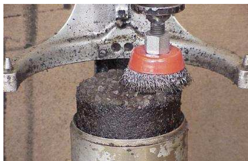
Figure 6 Setup for steel brush test
