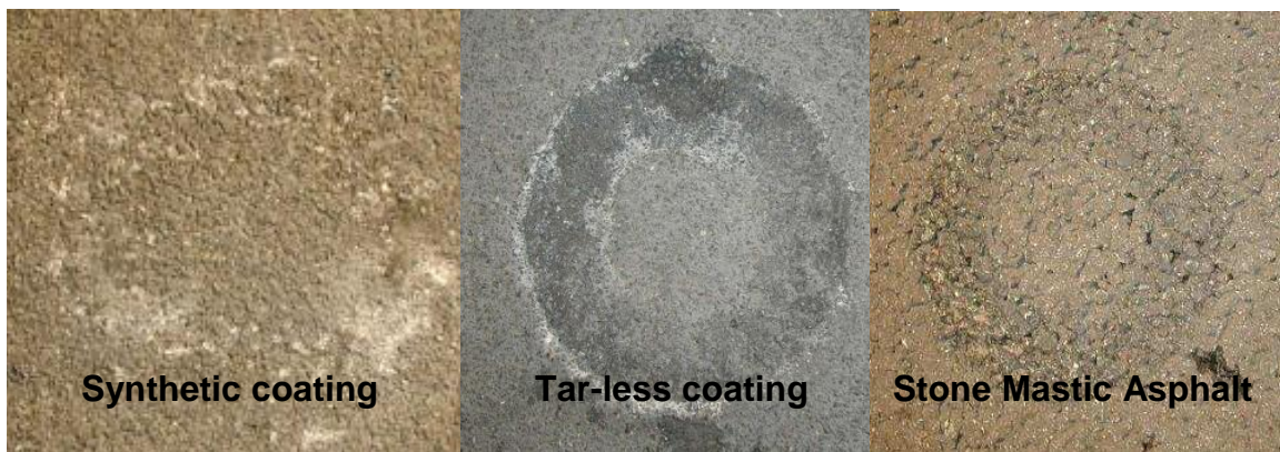
Figure 5 Results of raveling test on three kinds of coatings
