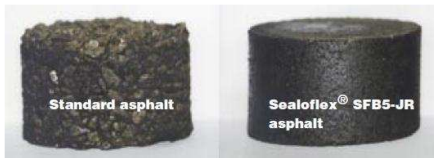
Figure 8 Compacted samples after 24 hours immersion in jet fuel
