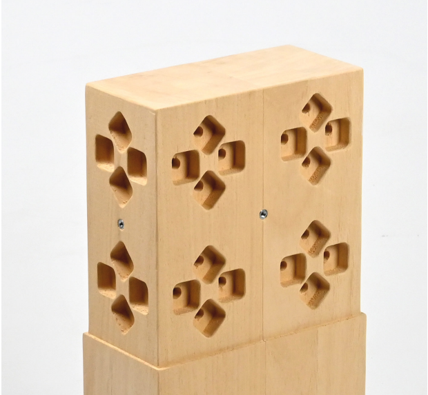
Figure 107. CNC milled sockets for nuts placement (by author 2023).
