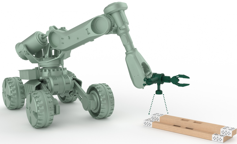
Figure 94. Robot computer vision and sensing checking the elements for calibration (by author, 2023).
