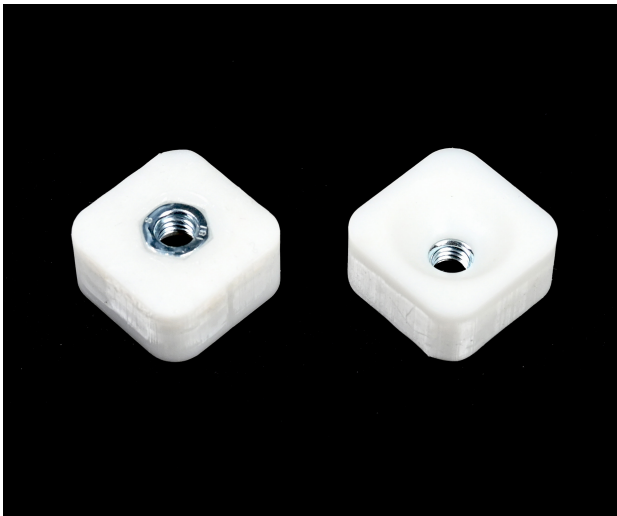
Figure 105. Resin 3D printed nuts with M6 nuts (by author 2023).
