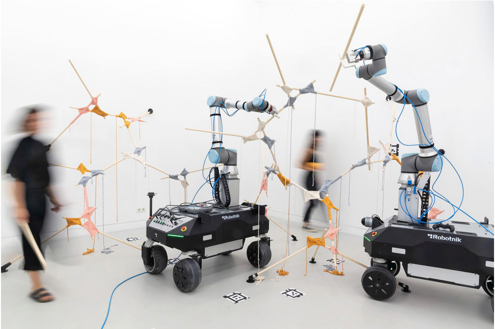
Figure 16. A cooperative proof-of-concept prototype has been developed to evaluate the design principles and workflow of an assembly cycle comprising five key components: interactive design, robotic assembly, manual assembly, rope jointing, and element tracking (Mitterberger, 2022).
