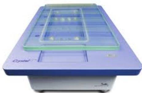
(a) The Crystal16, which allows for transmittance determination data for different temperature profiles. The can hold up to 16 vials in 4 temperature profile blocks, which can contain 4 vials each.
