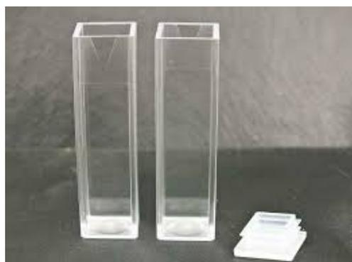
(a) The cuvettes and a sealing cap, which were used for the imaging experiments. The cuvettes were transparent with a thickness of approximately 1 mm.
