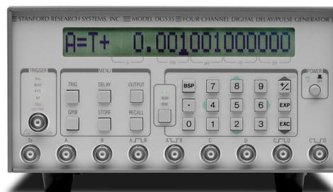
(b) The Stanford Research Systems Model DG535 digital delay / pulse generator which is used for triggering the recording of an image sequence. Full specifications can be found in the service manual [67].
