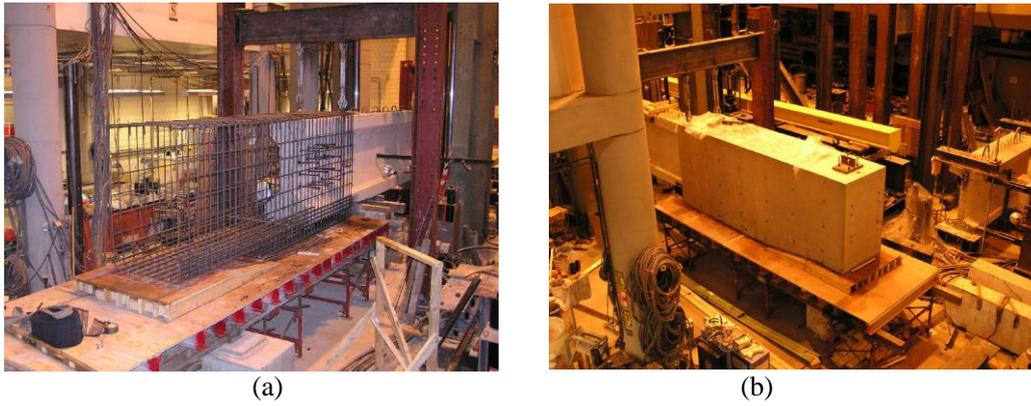
**Figure 4.3-3:** Extension construction (a) before casting, (b) after casting (Runzell et al. 2007)
