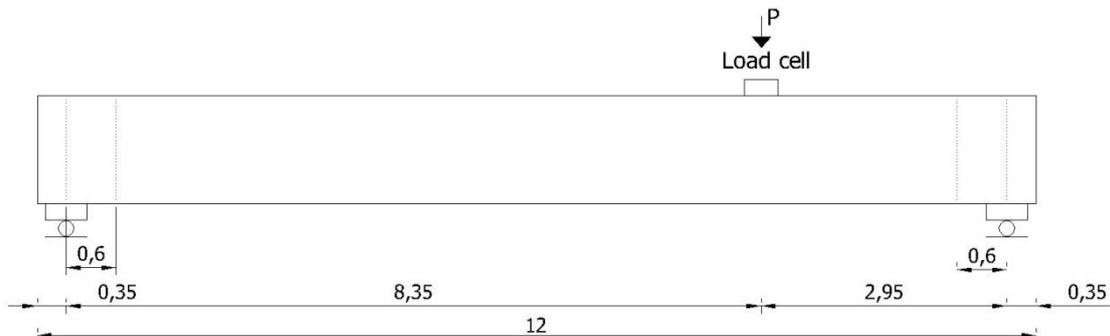
**Figure 5.1-4:** Case of DIANA User's Contest. Experimental test setup
