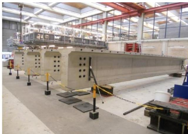
**Figure 5.1-1:** Case of DIANA User’s Contest. T-shaped prestressed girders tested in the Stevin Laboratory at TU Delft (picture given in the contest, [www.dianausers.nl](http://www.dianausers.nl))
