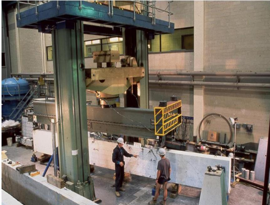
**Figure 3.2-3:** Case RB2. Experimental setup, (Collins and Kuchma 1999)
