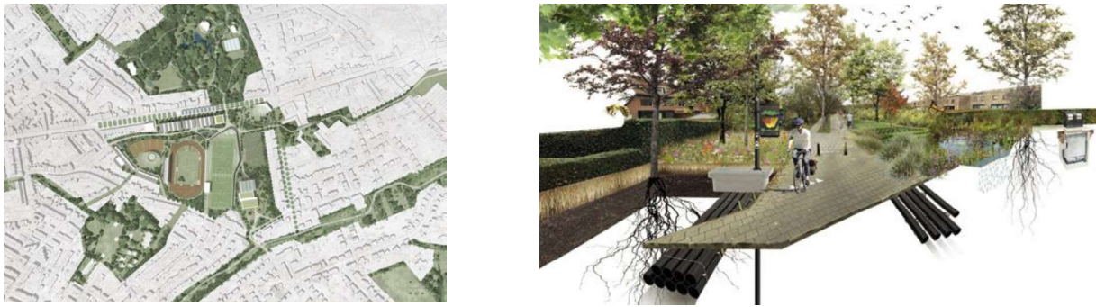
Figure 5 and 6. Leuven: Climate joints connect sport park and surroundings, and integrate eco-system services, and utilities. Cross-section of a Climate joint with integrated cycle route [16].
