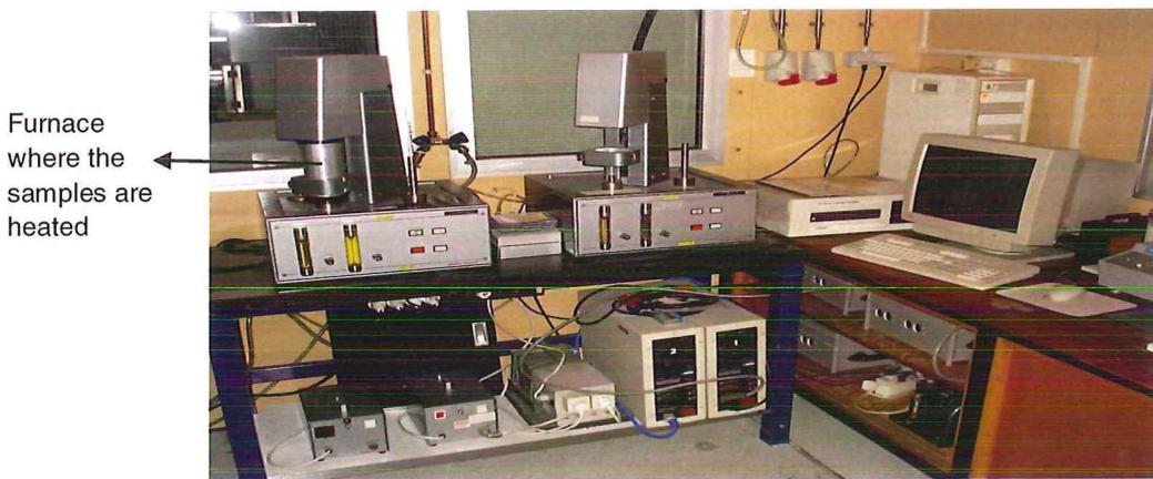
**Figure 2.5.** The differential scanning calorimeter used for the study.
