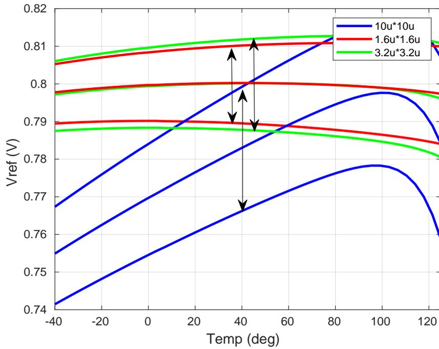
Figure 4.3:  $V_{ref}$  versus temperature for different emitter areas across FFFF, TTTT and SSSS corners
