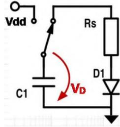
Figure 2.4: Capacitive bias of PN-junctions [8]
