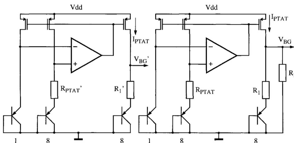
Figure 2.1: Conventional and low supply voltage bandgap circuits [15]
