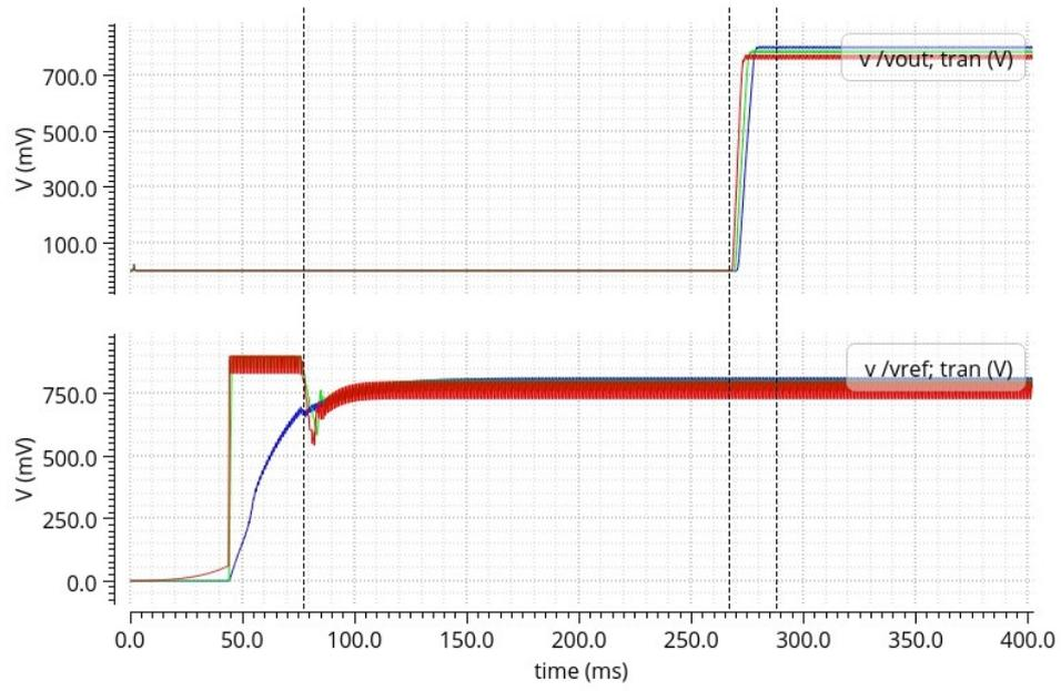
Figure 5.11: Transient  $V_{ref}$  and  $V_{out}$  in FFFF125 (red), TTTT27 (green), SSSS-40 (blue)
