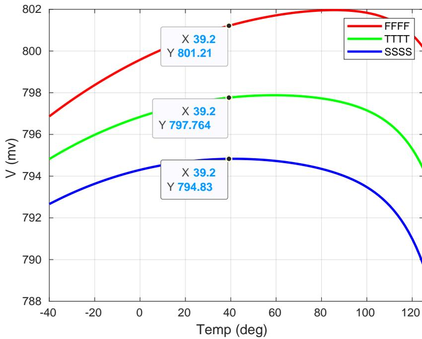
Figure 4.7: Error contribution on  $V_{ref}$  with corner spreads in  $R_{PTAT}$ ,  $R_{CTAT}$ , and  $R_{ref}$ .
