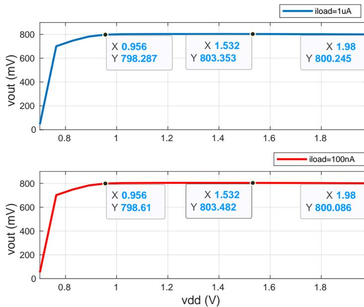
Figure 5.5: LDO output voltage versus input voltage ( $V_{dd}$ ) for maximum and minimum load currents.
