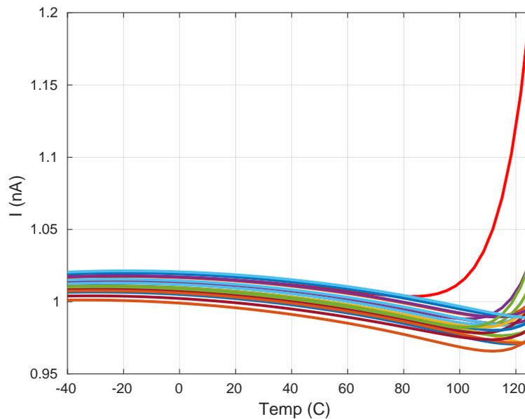
Figure 4.14: Bandgap current with and without (red) compensation.
