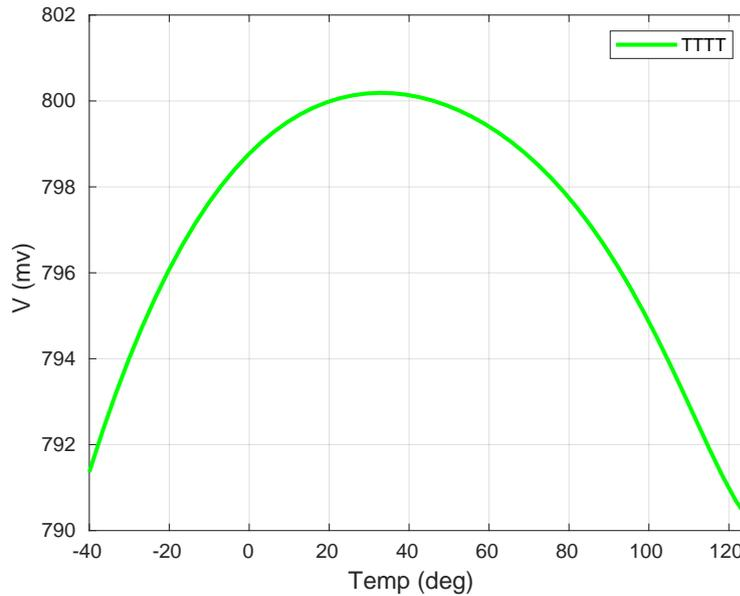
Figure 4.12: Bandgap reference voltage after removing Rs
