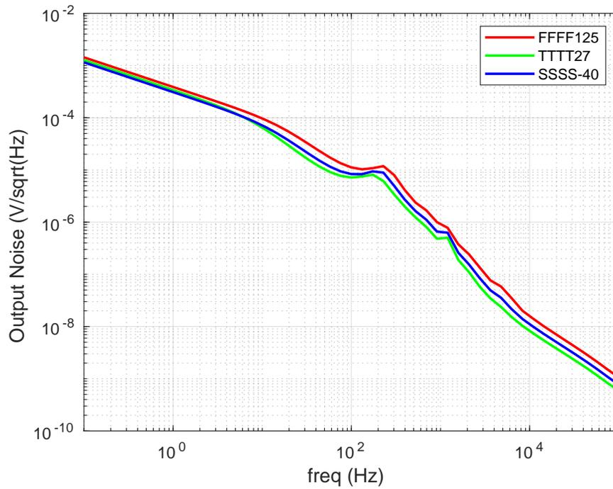
Figure 4.29: Output voltage noise density of bandgap reference
