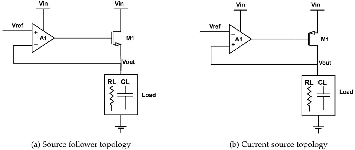
Figure 5.2: Pass transistor topologies: (a) Source follower, (b) Current source
