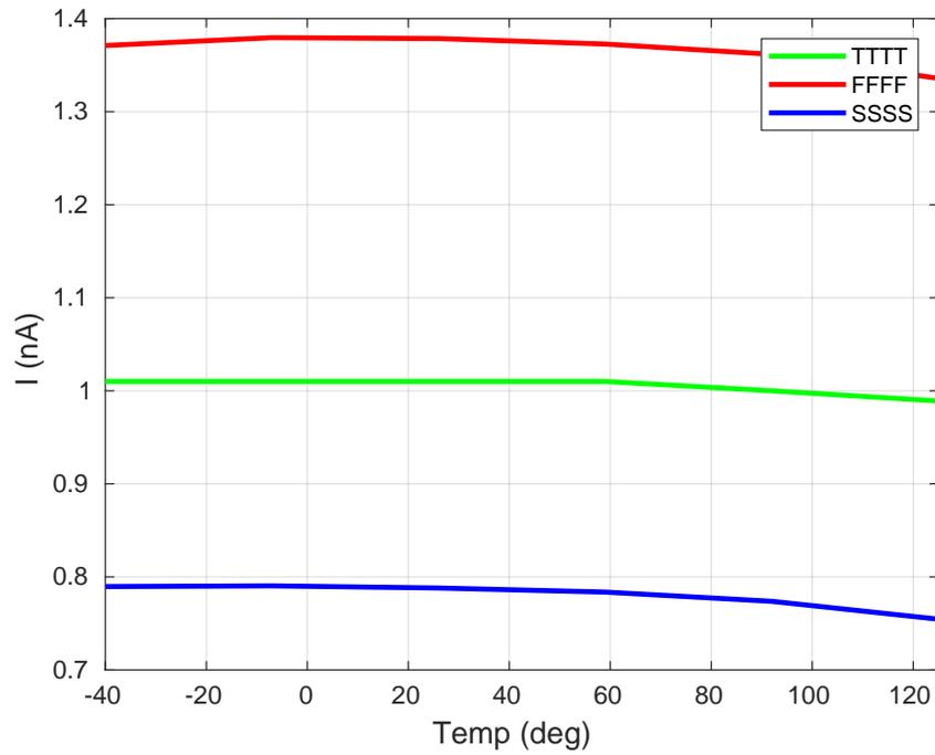
Figure 4.23: Output current over the temperature range for different process corners
