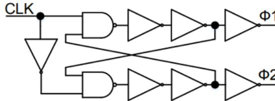
Figure 3.4: Schematic of the cross-coupled RS flip-flop
