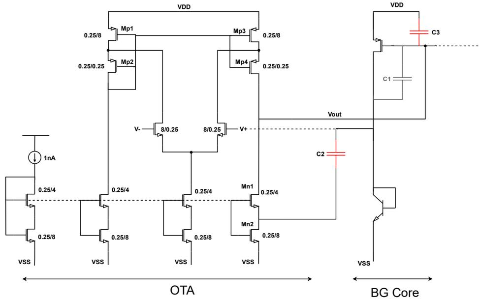
Figure 4.9: Schematic of the pseudo-folded cascode OTA with transistor sizes and compensation capacitors.
