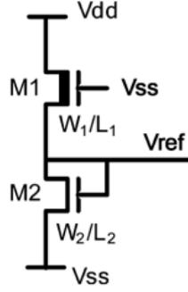
Figure 2.7: Two transistor (2T) voltage reference [22].
