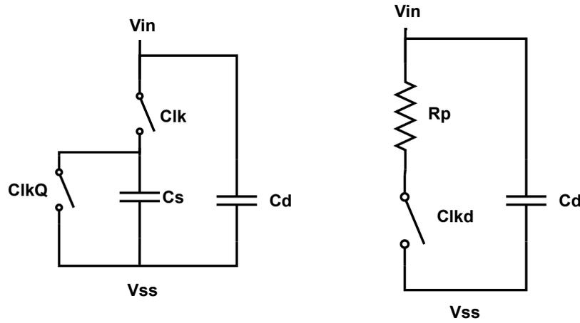
Figure 4.15: Switched capacitor resistor (left) and duty-cycled resistor (right)
