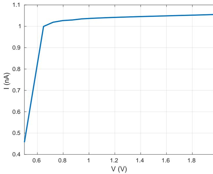
Figure 3.6: Average output current versus supply voltage
