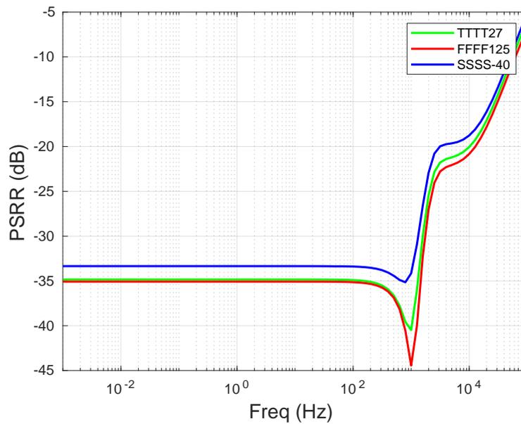
Figure 3.7: PSRR curves of output current
