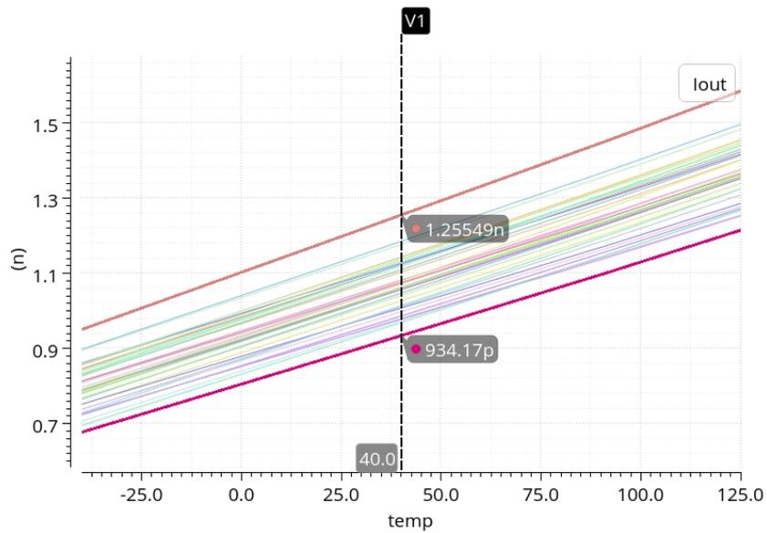
Figure 3.12: Monte Carlo simulation results for the output current over temperature
