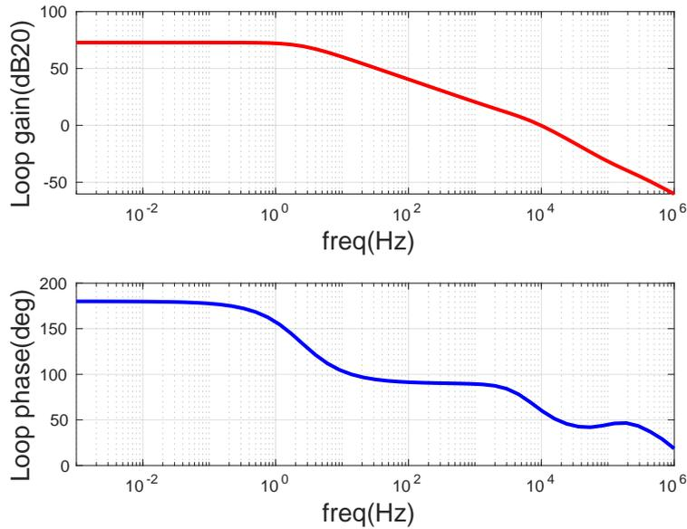
Figure 4.10: Stability analysis of pseudo folded cascode OTA in closed loop bandgap core
