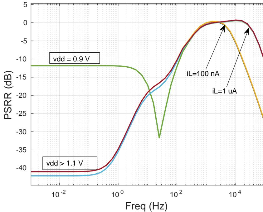
Figure 5.6: PSRR curves for different supply voltages and load currents
