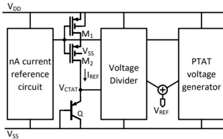
Figure 2.6: Proposed ultra-low-power voltage reference architecture in [7]
