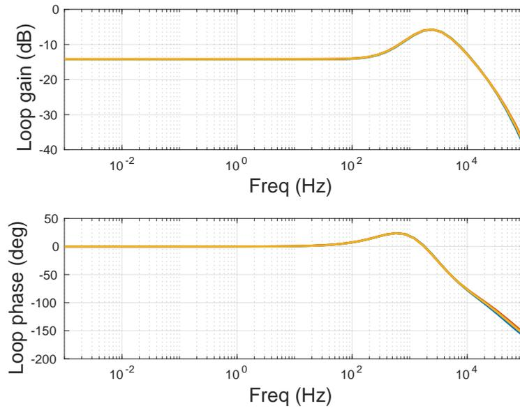
Figure 3.8: Frequency response of the PTAT closed loop.
