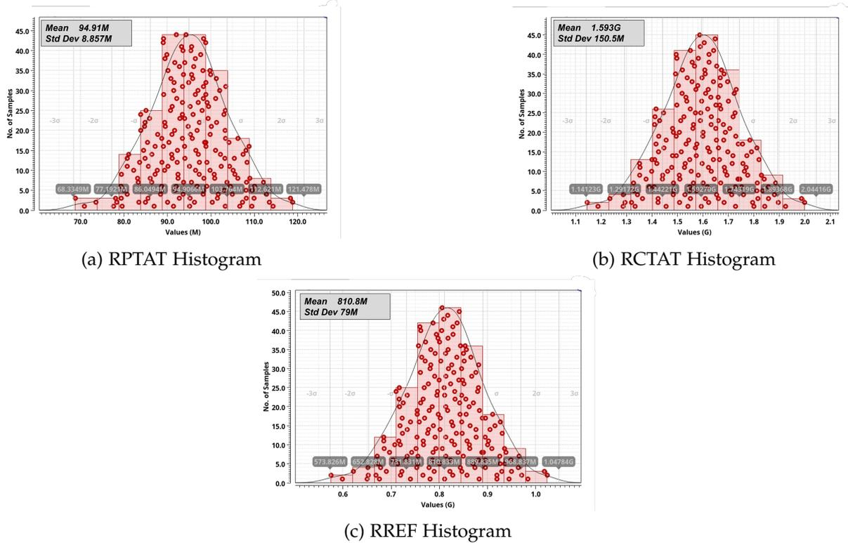
Figure 4.32: Monte Carlo simulation results for the duty-cycled resistors: (a) RPTAT, (b) RCTAT, and (c) RREF histograms.
