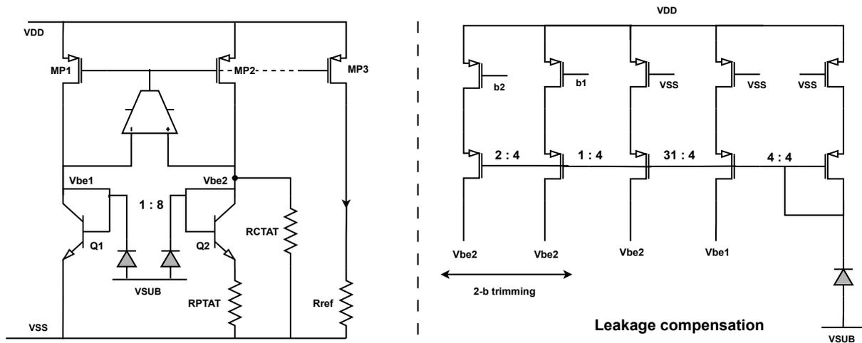
Figure 4.13: Parasitic diode leakage compensation circuit, dummy diode is generated in the layout with a DNW layer on top of the P-substrate
