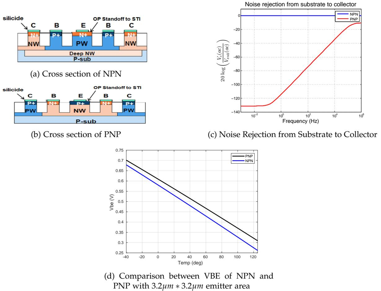
Figure 4.2: Comparison of NPN and PNP cross sections, noise rejection characteristics and base-emitter voltages
