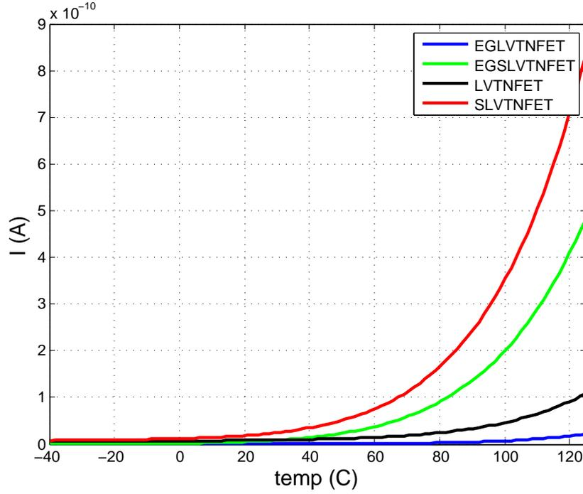
Figure 3.1: Channel leakage current as a function of temperature for unit transistors ( $\frac{W}{L} = \frac{1\mu}{1\mu}$ )
