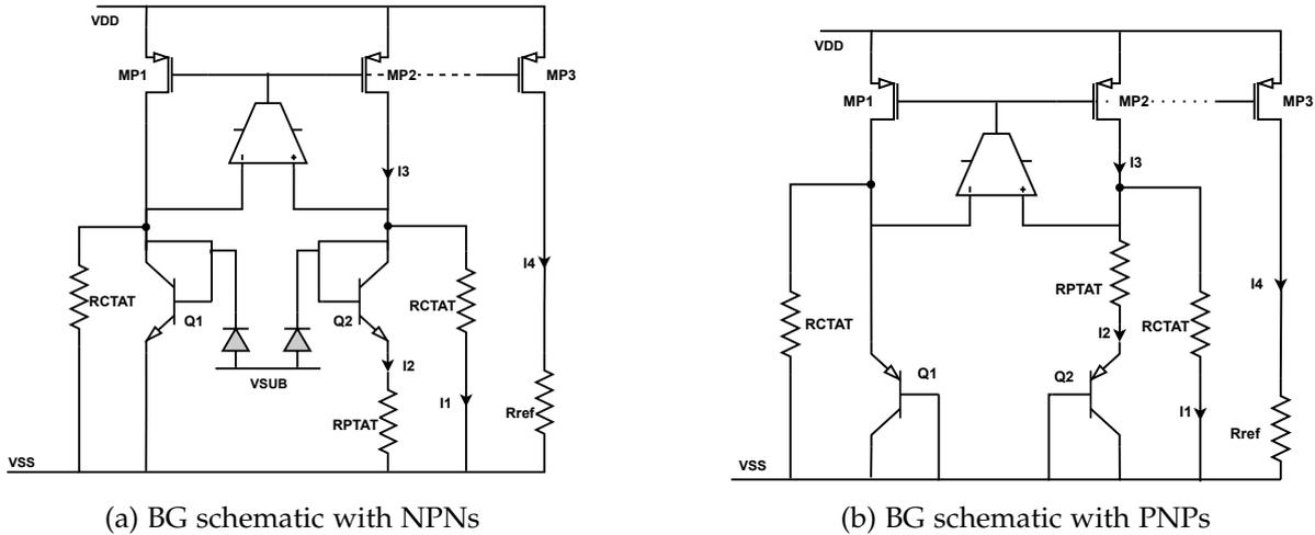
Figure 4.1: Comparison of BG schematic with NPNs (a) and PNPs (b)
