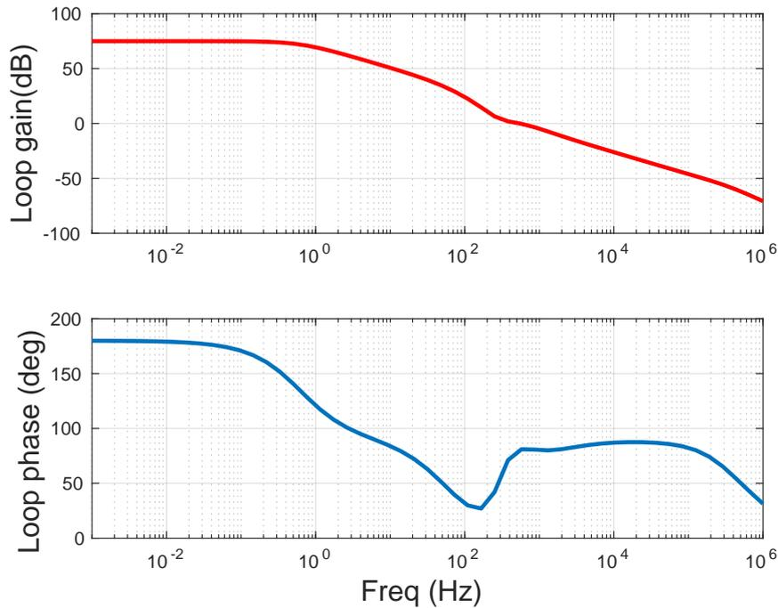
Figure 4.18: Stability results of the bandgap loop after adding parallel capacitors.
