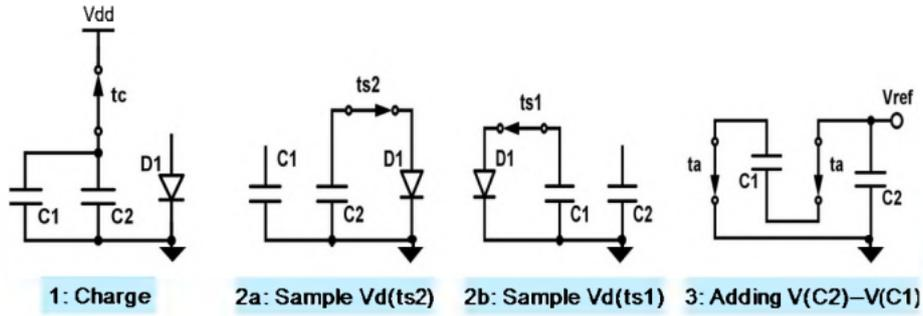
Figure 2.5: Capacitive switching phases to generate  $V_{ref}$  [8]
