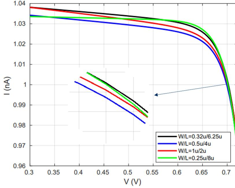
Figure 4.5:  $I_d$  of PMOS mirror vs  $V_S$  with different transistor sizings
