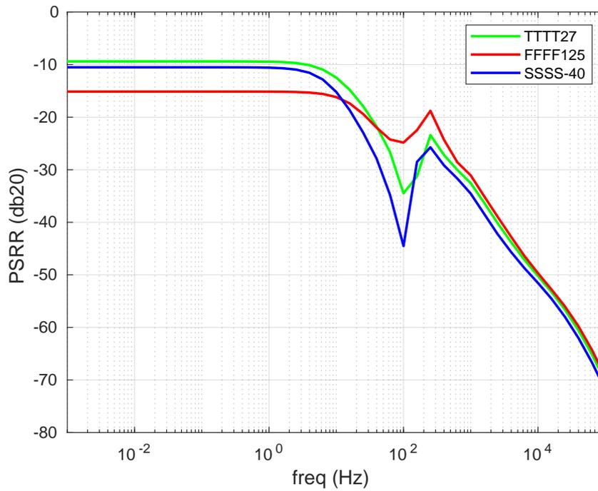
Figure 4.26: PSRR curves for different process corners
