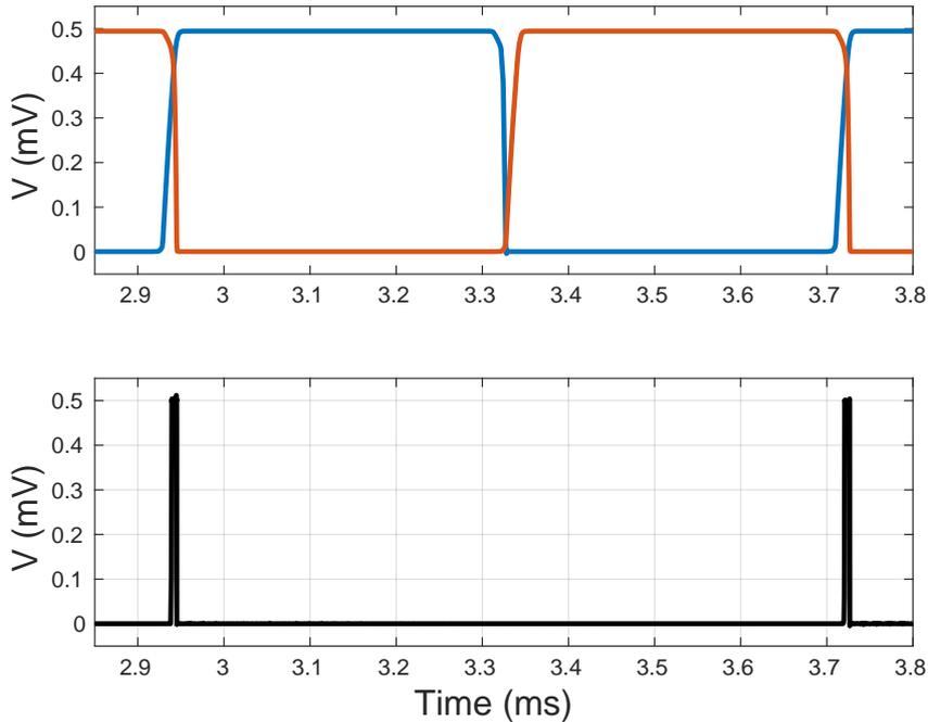
Figure 4.17: Ring oscillator two consecutive clock signals and the final clock with 1% duty cycle
