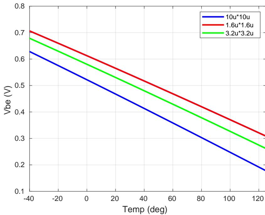
Figure 4.4:  $V_{BE}$  versus temperature for different emitter areas
