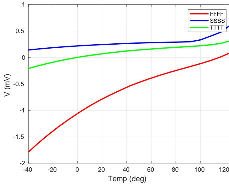
Figure 5.4:  $V_{ref} - V_{out}$  over temperature range and process corners
