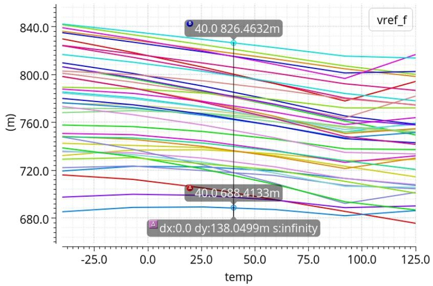
Figure 4.30: Monte Carlo simulation results for the reference voltage over temperature
