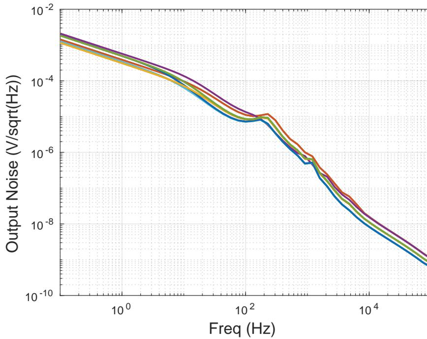
Figure 5.8: Output voltage noise density of LDO
