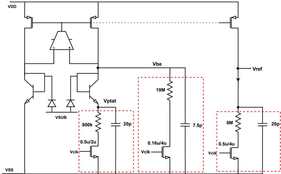
Figure 4.19: Bandgap schematic with optimized switch sizes and parallel capacitor values.
