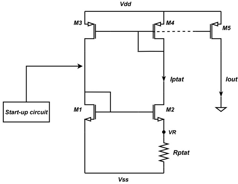
Figure 3.2: PTAT Current Reference Schematic
