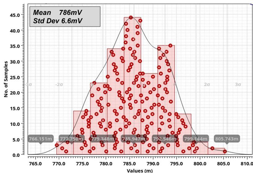
Figure 5.9: Monte Carlo simulation results for the LDO output voltage.
