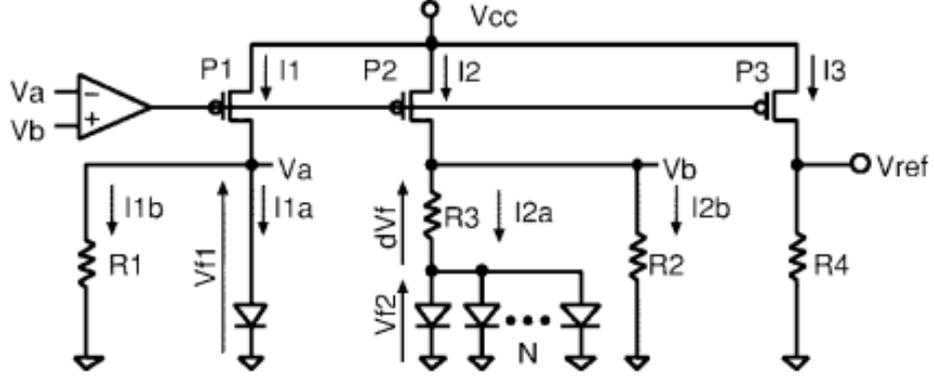
Figure 2.3: Schematic of the current and voltage reference with PTAT and CTAT currents [3]
