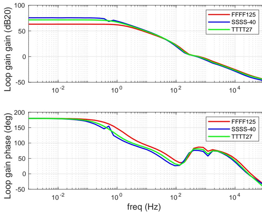
Figure 4.27: Bandgap core loop stability analysis in different process corners
