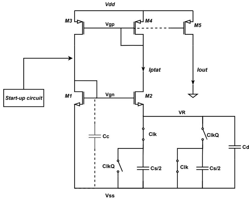
Figure 3.3: Schematic of PTAT current reference with switched capacitor resistor
