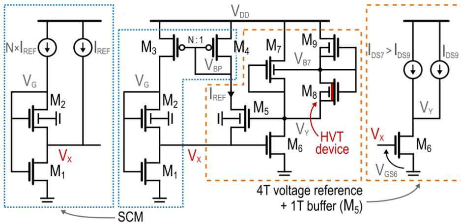
Figure 2.10: Schematic of the current reference with SCM and 4T voltage reference [12]
