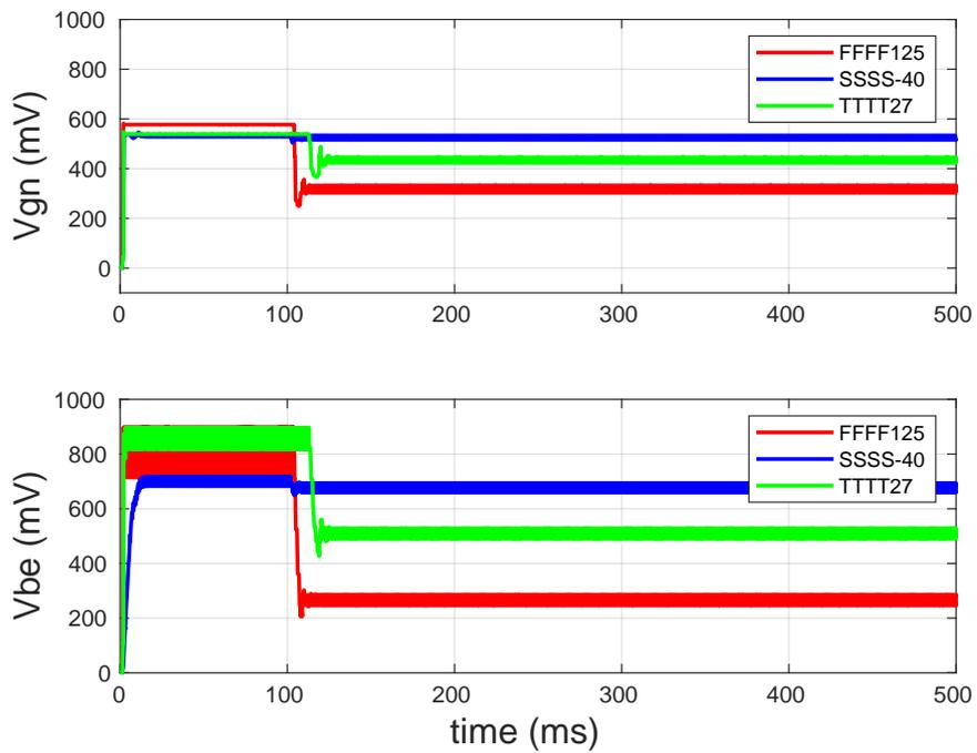
Figure 4.21: Transient response of  $V_{be}$  and  $V_{gn}$
