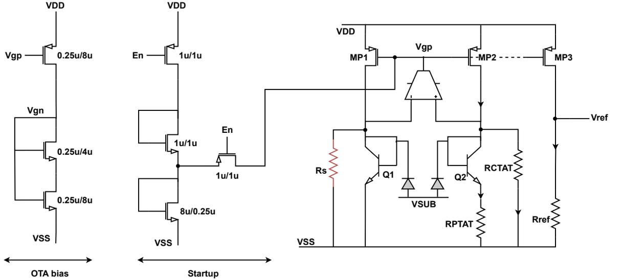
Figure 4.11: Schematic of the bandgap reference circuit with side resistor ( $R_s$ ) and the proposed startup circuit
