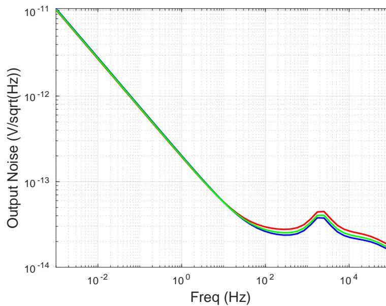
Figure 3.10: Output current noise density of PTAT reference
