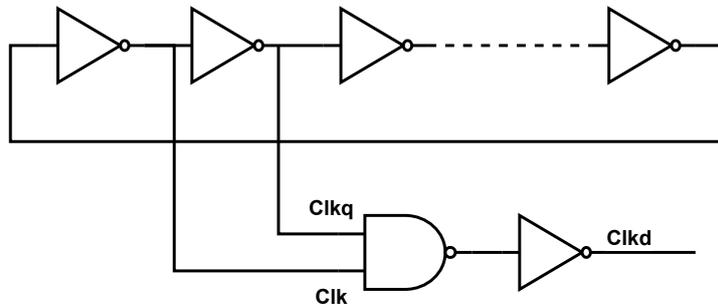
Figure 4.16: Ring oscillator with 51 inverters to generate 1% duty cycle
