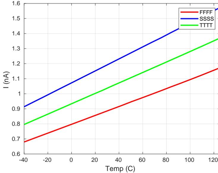
Figure 3.5: Output current over the temperature range for different process corners
