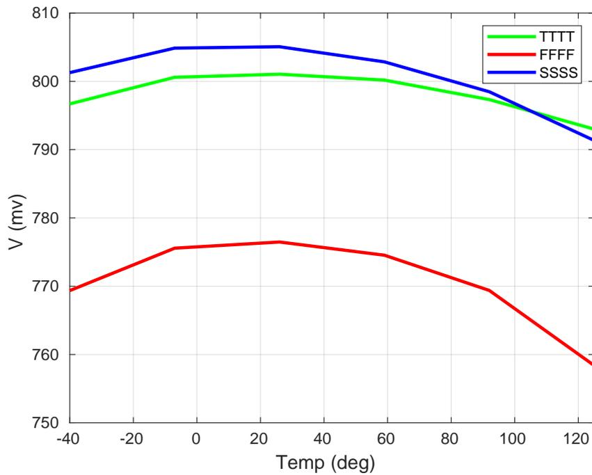
Figure 4.24: Bandgap voltage reference over the temperature range for different process corners
