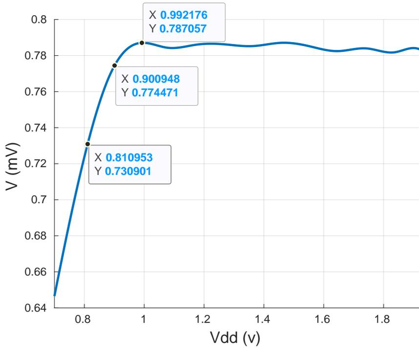
Figure 4.25: Reference voltage variation over the supply voltage
