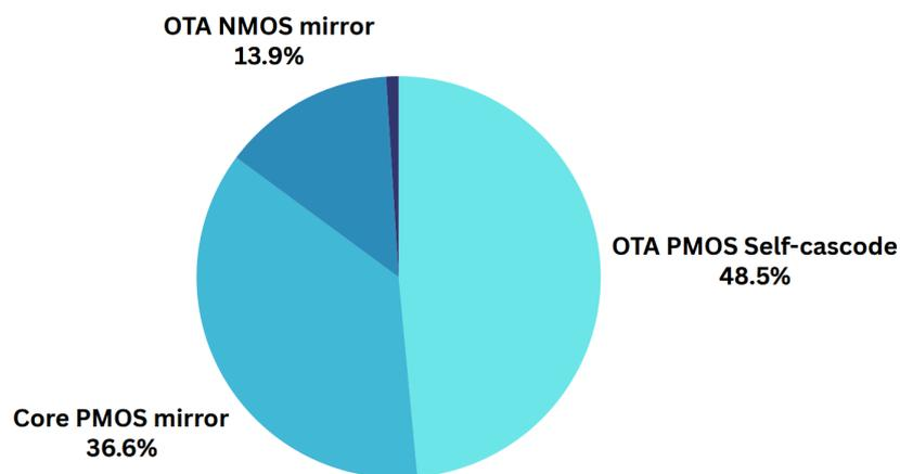
Figure 4.28: Pie chart of the main noise contributors to bandgap reference voltage
