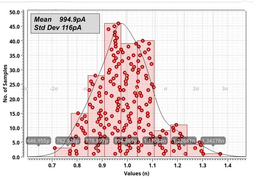
Figure 4.31: Monte Carlo simulation results for the output current.
