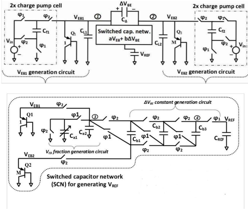
Figure 2.2: Bandgap reference circuit using charge pumps and a switched capacitor network [23].
