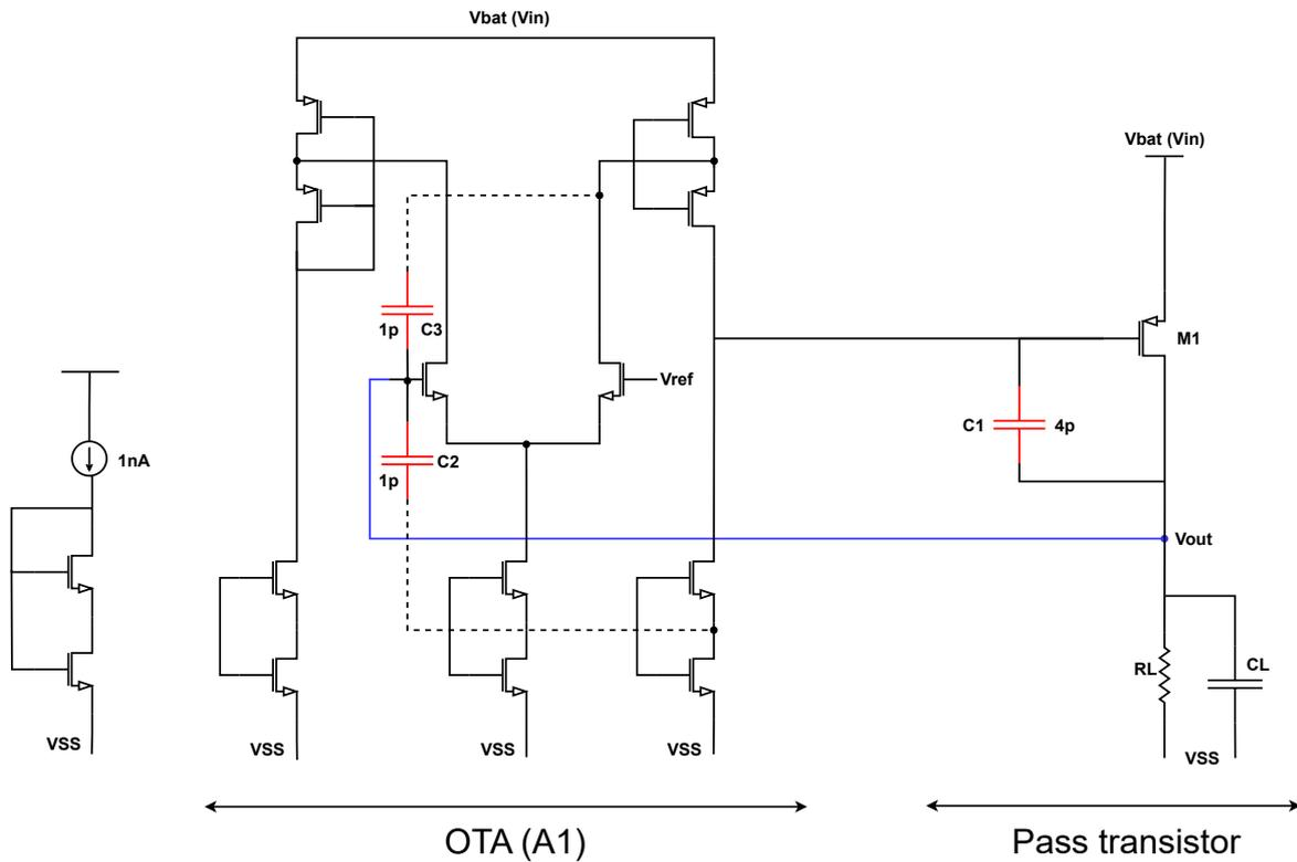
Figure 5.3: LDO schematic with capacitor values used for optimal stability.
