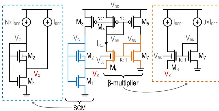
Figure 2.9: Self-cascode MOSFETs used for nA-range reference current generation [13]
