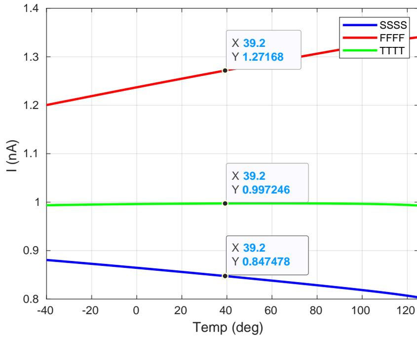
Figure 4.6: Effect of  $R_{PTAT}$  corner spread on reference current
