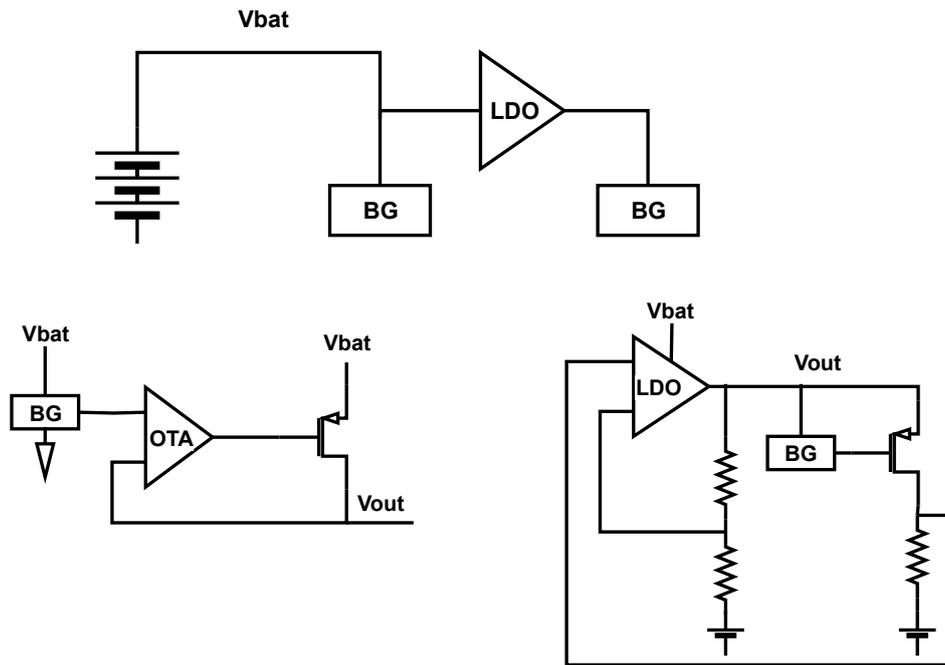
Figure 5.1: System-level options for integrating bandgap reference and LDO
