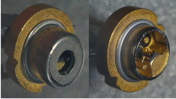
Figure 5.1: Figure depicting a normal laser diode and a de-canned laser diode
