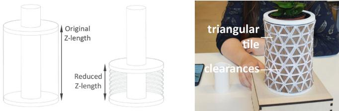
**Fig. 1.** Z-length reduction – tessellated triangular design
