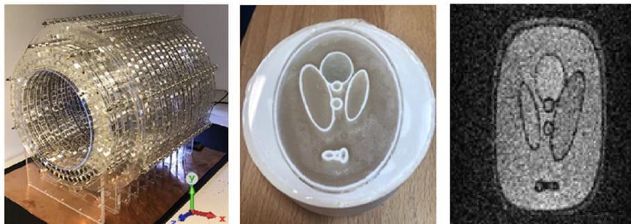
**Fig. 2** (Left) A low-cost portable MRI at LUMC, (Middle) The 3D printed phantom (Shepp Logan) and (Right) The image of the 2D phantom acquired using the Low-Field MRI scanner on the left
