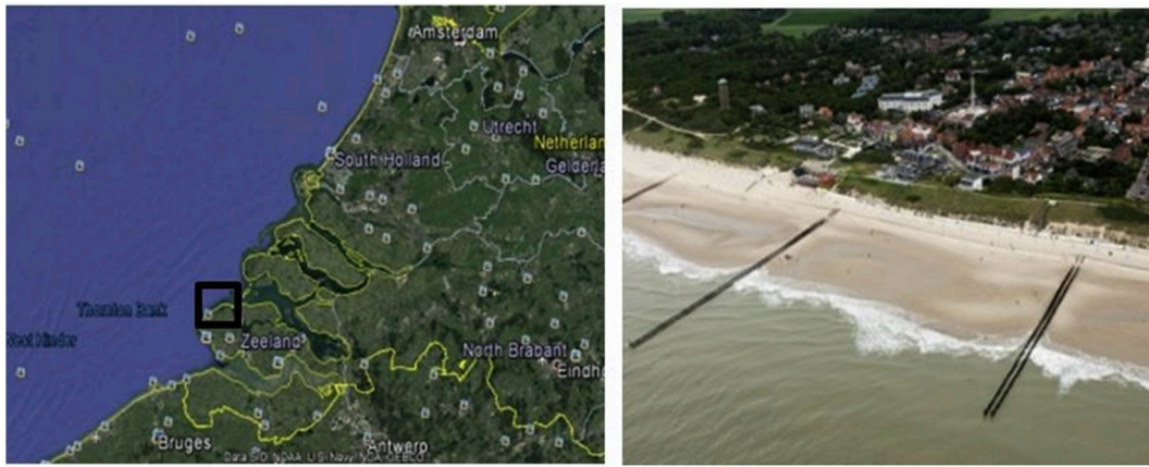
Fig. 1. Left: The location of a pile groin engineered coast in Zeeland Province, The Netherlands (in the black rectangle, from Google earth); right: the continuous straight shoreline response to PPGs at the coast (source: https://beeldbank.rws.nl , Rijkswaterstaat).
