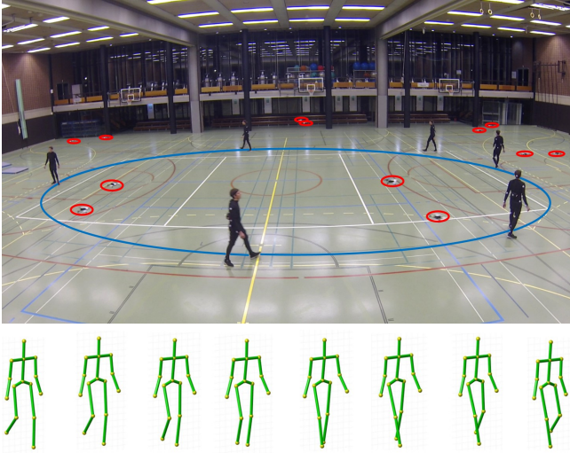
Fig. 8. Experiment 3: Top: Subject walking over a long distance and time period in circles - indicated in blue - with a walking speed around 1.5 \frac{m}{s} (top). The drones follow the subject and always position themselves to optimally observe the markers, mounted on the back of the subject. Bottom: reconstructed gait cycle recorded during the experiment.
