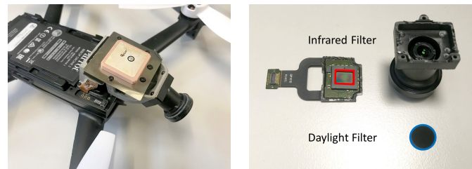
Fig. 5. The active marker detection scheme only requires little modification to the Parrot Bebop's hardware and is hence cheap. First, the lens-mount has to be removed using a heat-gun (left). Then, the infrared filter (red) can be removed and the daylight filter (blue) can be fitted to the lens mound. In the last step, the camera has to be reassembled and re-calibrated.
