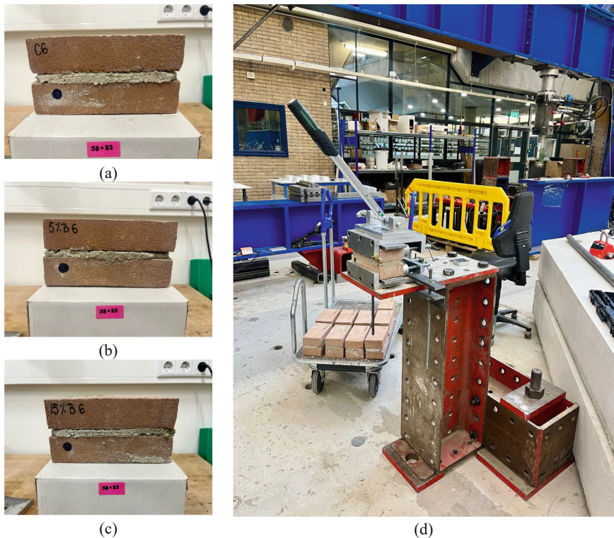
Fig. 1. (a) Reference and bacteria-based masonry couplets at agent concentrations of (b) 5% and (c) 15%; (d) bond wrench test set-up used for testing.
