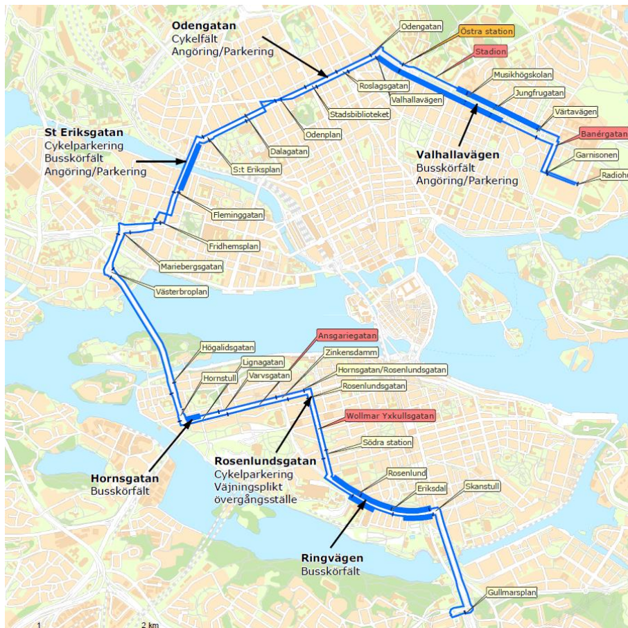
Fig. 5 Physical measures that were implemented during the trial period (cancelled stops in red and new bus lanes in bold blue, other measures included removed parking lots and changes in bike lanes)
