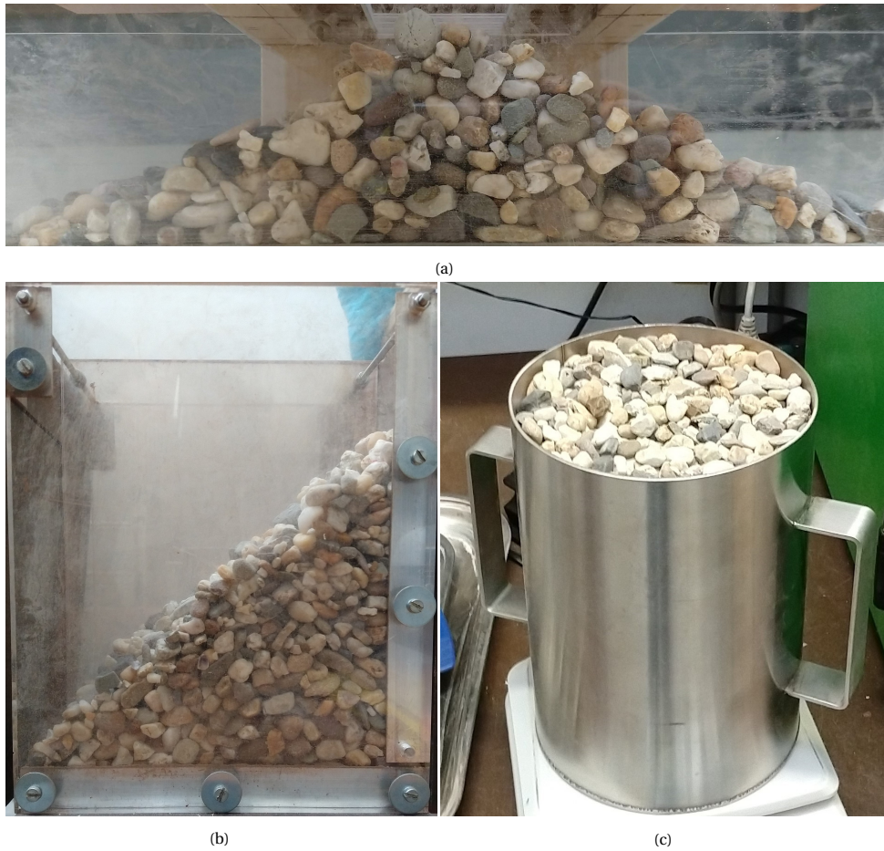
Figure 4.1: Laboratory scale tests (a) Pile forming test (b) Ledge test (c) Bulk density test
