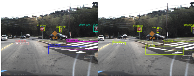
Figure 9. Shows how different class labels are grouped together such that each action of the application is done based on only 1 prediction of a super-class. Picture is taken from dataset used in the experiment but manually labelled to include extra classes to show as example. Left is what the labelling would look like if base classes were used. Right is what the labelling would look like if the classes were grouped.
