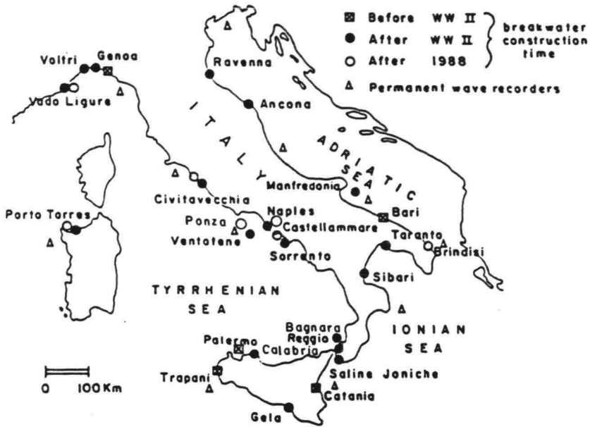
FIG. 1: Location map of vertical breakwaters in Italy (1992)
