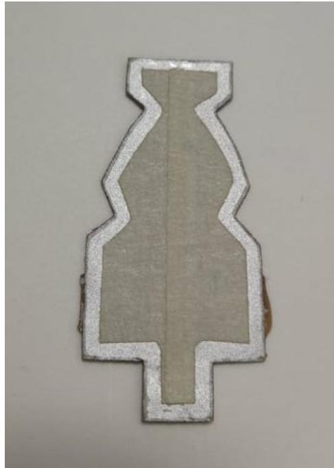
Figure 2.5: Sensors with edge cleaned from silver layer. Version 2, larger offset of 2mm shown in figure. This offset width was enough to clean the sensor edge properly and therefore prevent short circuit. The simpler shape of the second version of the sensor also helped in the edge cleaning.
