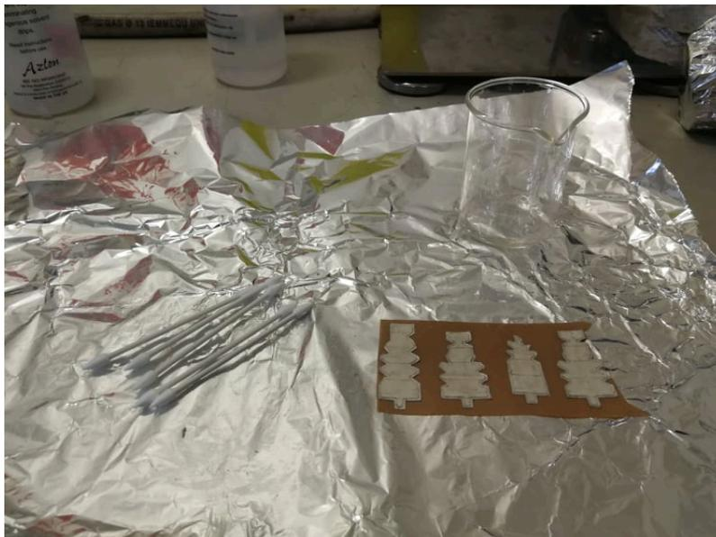
Figure 2.3: Setup for cleaning the sensors' offset from the silver layer to prevent short circuit. On the top right a baker with acetone to remove the silver layer using cotton-swabs shown on the left. The sensors covered with paper tape in the central part to protect the rest of the silver from the acetone, get cleaned in the outer edge offset.
