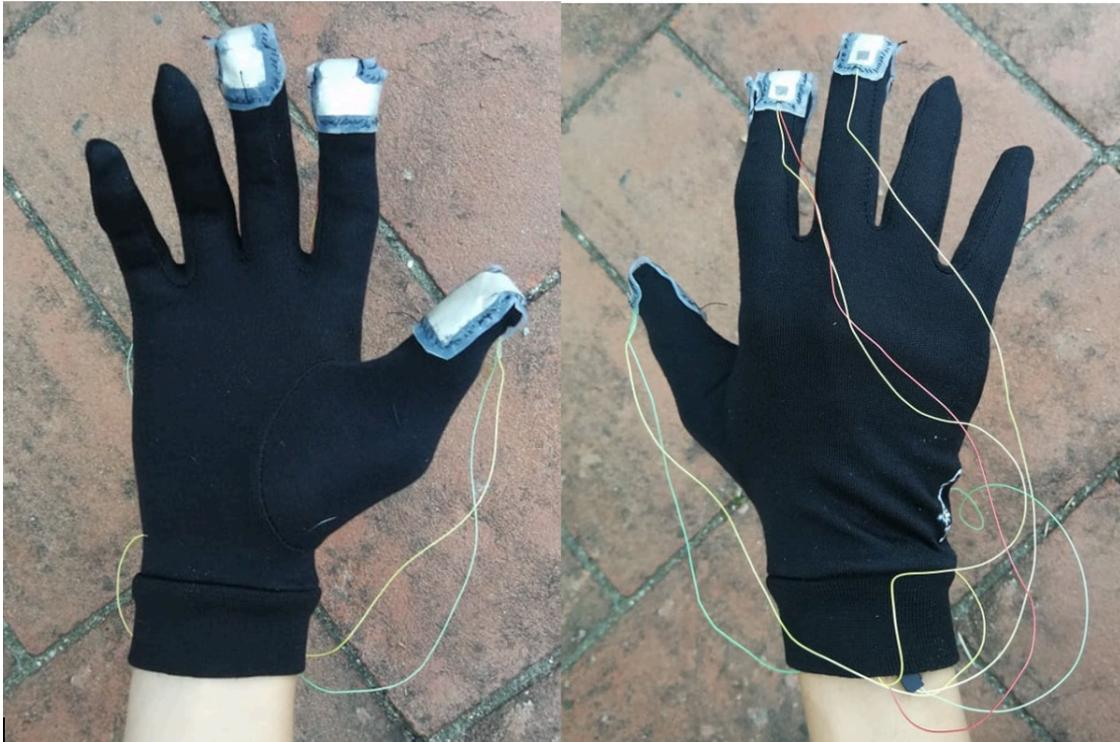
Figure 2.9: DESC glove, three sensors sewed at the fingertips one on the thumb, one on the index and one on the middle finger. The sensors were sewed using the silicone layer offset to the fabric of the glove. They were then covered with another layer of fabric, as shown in 2.10.
