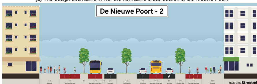
(b) The design alternative 2 for the normative cross-section of De Nieuwe Poort
