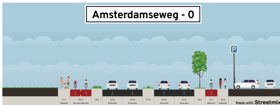
Figure 7.5: The current situation on the normative cross-section of the Amsterdamseweg
