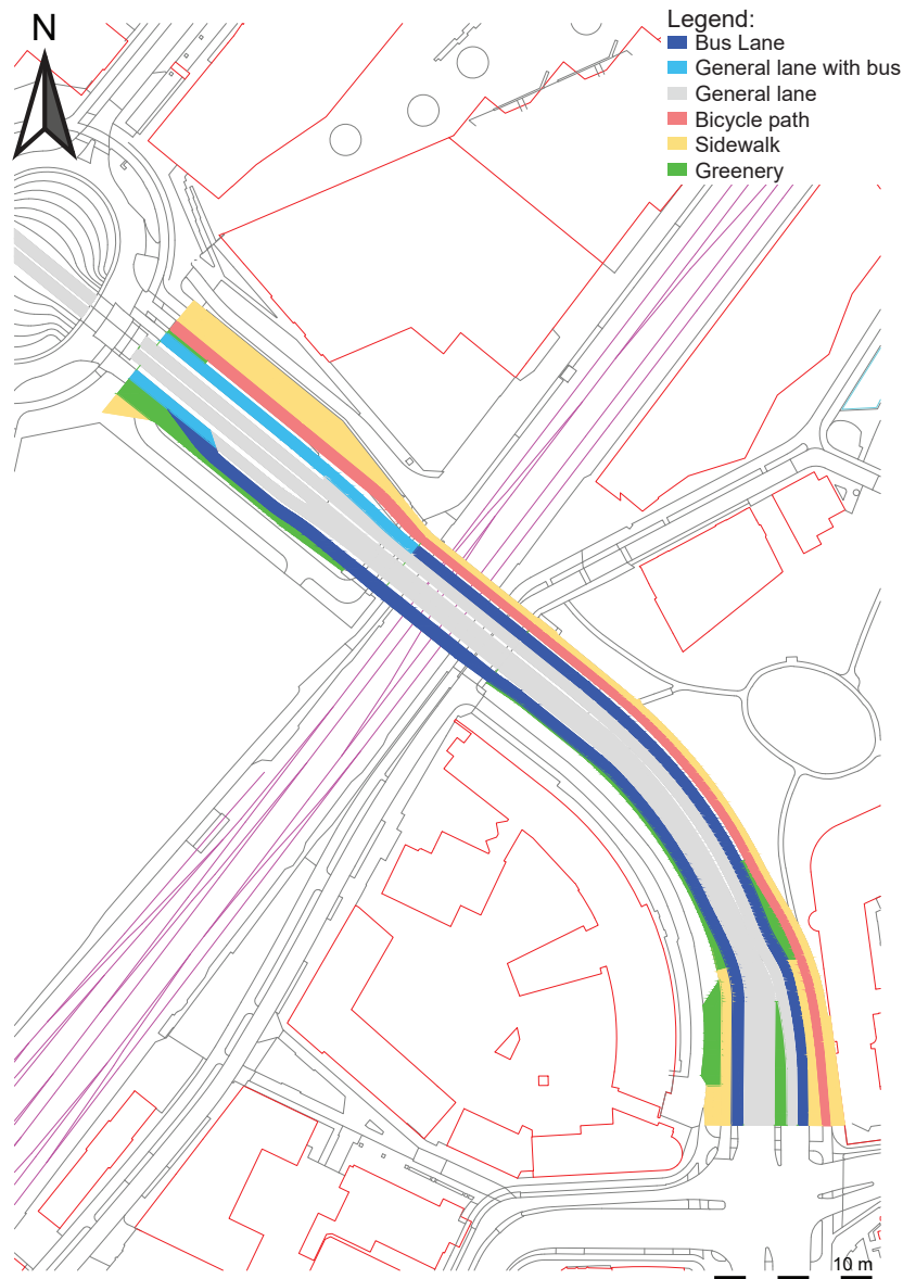
Figure 8.7: Design variant curb-side between the start at the Stadsring and the roundabout at De Nieuwe Poort
