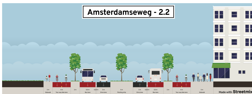
Figure 8.6: Design variant of the Amsterdamseweg on which design variant curb-side for design section Amsterdamseweg is based
