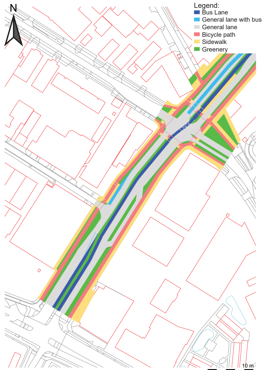
Figure 8.11: Design variant mostly median between the intersection with the Amsterdamseweg and the Koppelbridge
