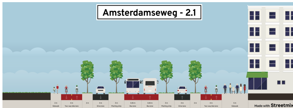
Figure 8.2: The design variant of the Amsterdamseweg on which the design variant median for the design section Amsterdamseweg is based
