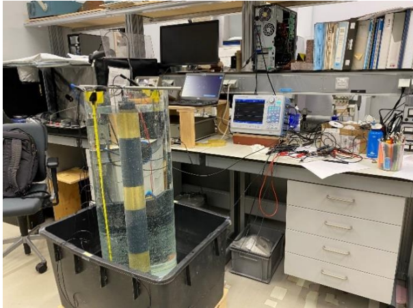
Figure 1 Prototype capacitive sensor in a water tank in the laboratory of the TU Delft.
