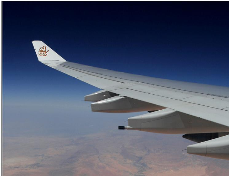
**Figure D.2:** Conventional winglet of an Airbus A340-541. Photo by Fabian Gysel. Equivalent to figure (3.7).
