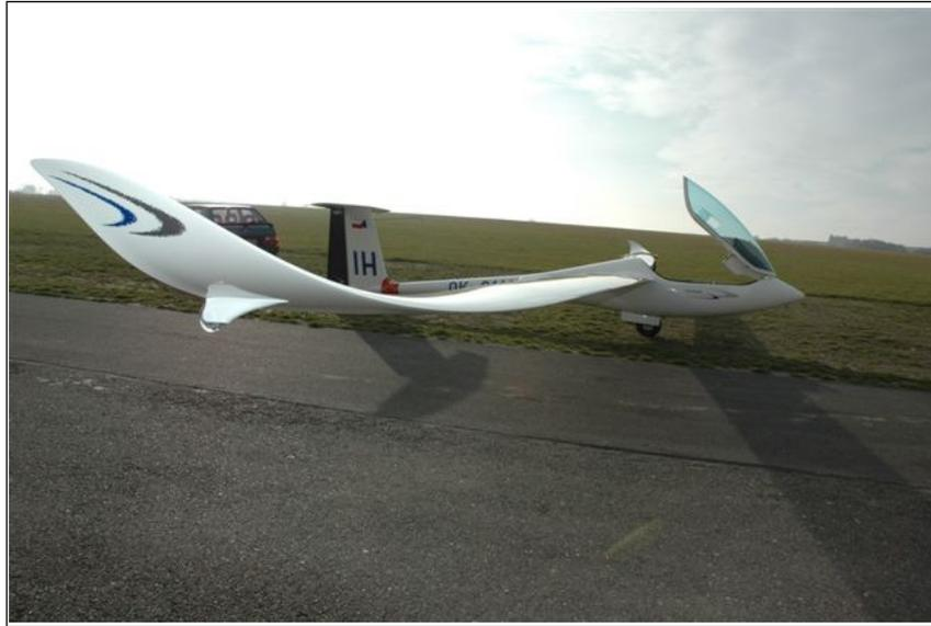
**Figure D.3:** Shark fin tip on a HPH 304 S sailplane. Photo by Tim Mara. Equivalent to figure (3.9).
