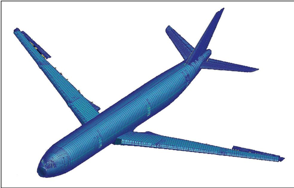
*Figure 6.12: Full (structural) model of the aircraft.*
