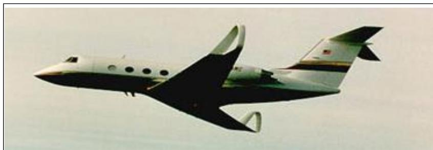
**Figure 3.3:** Spiroid wing tip. Picture by courtesy of Aviation Partners, Inc.
