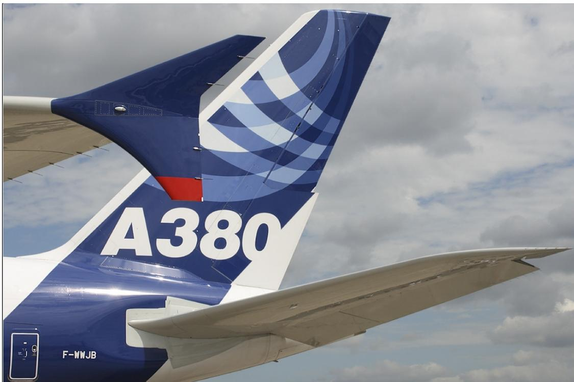
**Figure 3.10:** Wing Tip Fences on the Airbus A380. Photo by Thomas Wirtenberger. See figure (D.4) in the appendix for the full color image.
