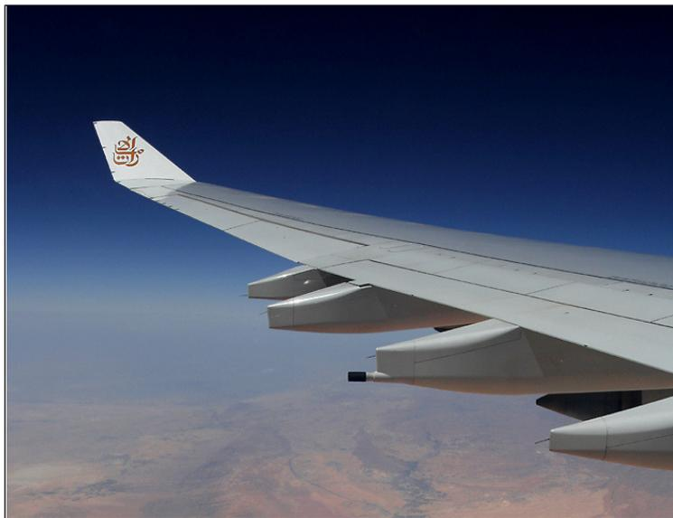
*Figure 3.7: Conventional winglet of an Airbus A340-541. Photo by Fabian Gysel. See figure (D.2) in the appendix for the full color image.*
