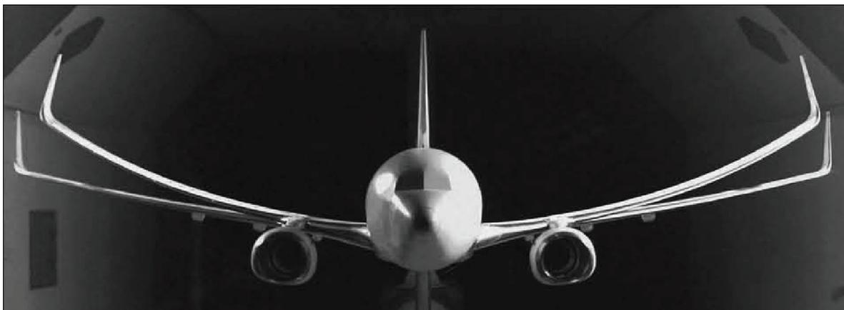
**Figure 3.11:** Image of the Boeing 737 wind tunnel model constructed in the shape of the 2.5g deflected wing superimposed over an image of the wing in the nominal 1g cruise shape. Picture by courtesy of the Boeing Company
