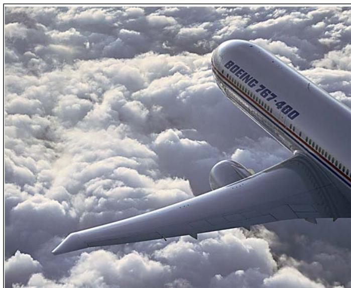
*Figure 3.8: Raked tip on a Boeing 767-400ER. Picture by courtesy of the Boeing Company*
