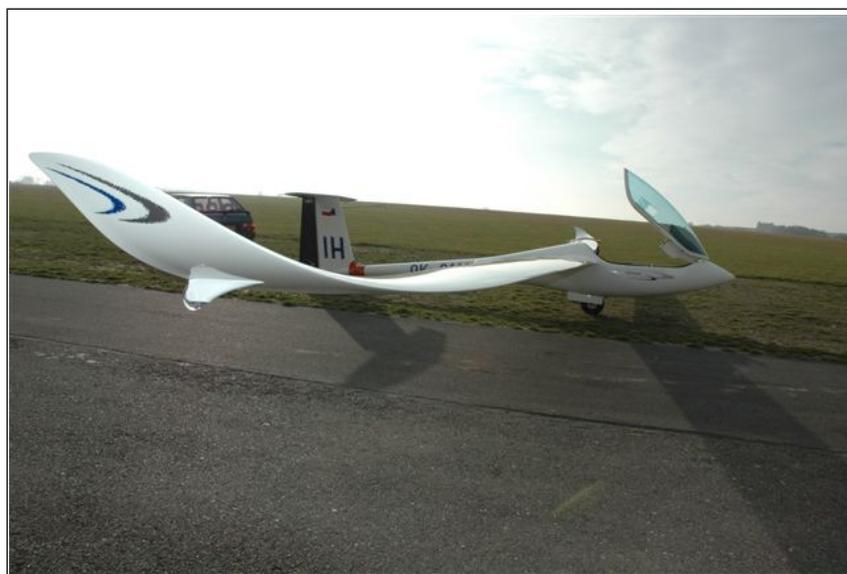
*Figure 3.9: Shark fin tip on a HPH 304 S sailplane. Photo by Tim Mara. See figure (D.3) in the appendix for the full color image.*
