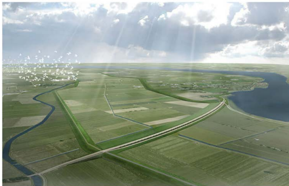
Bird-eye view impression of the high water bypass channel and new dike boundary. Polder landscape is preserved.
