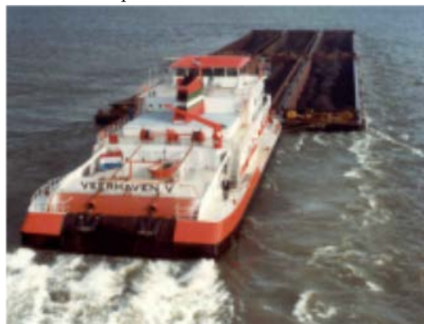
6-barge push-tow unit CEMT-class VIIa
