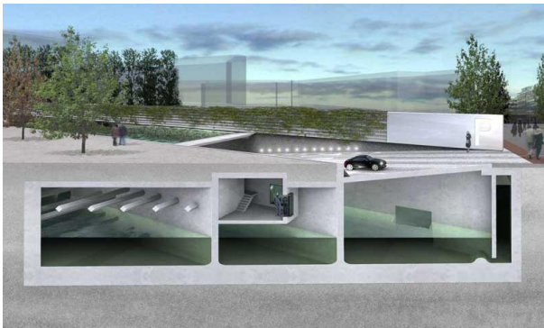
Figure 4.21 Using parking garages for stormwater storage
