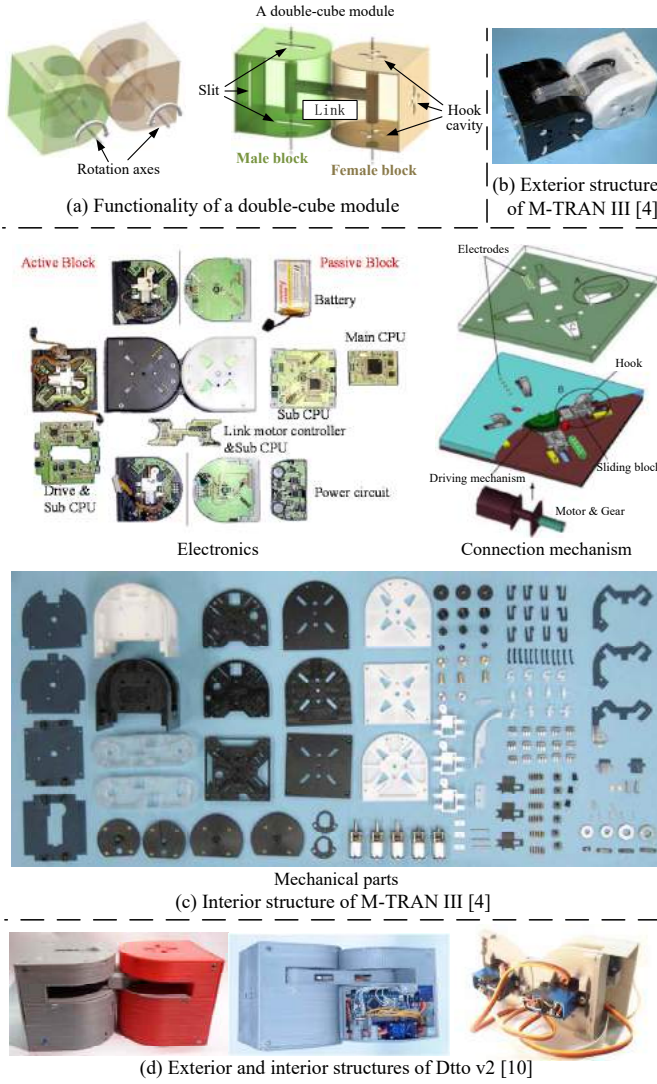
Fig. 1. All self-reconfigurable robots using double-cubic modules have similar exterior structures and similar functions that: each module consists of two semi-cylindrical boxes and a link, and each box can rotate independently around its axis by \pm 90^\circ (see (a) for the design of our EasySRRobot). The male box (in green color) has slits on its three faces, and the female box (in yellow color) has hook cavities on its three faces. The double-cube modules used in M-TRAN III (see (b) and (c)) and Dtto v2 (see (d)) have different interior structures for placing on-board components, which lead to different placements of the link – the link of Dtto is placed closer to one side of the box than the other side.
