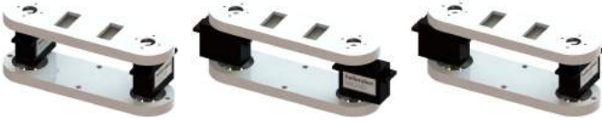
Fig. 5. Examples of possible orientations of two HX1218D servomotors for driving the link. Rotation axes of servomotors coincide with the rotation axes of boxes, and the link connecting two servomotors must be perpendicular to rotation axes. In our design, the link is hollowed such that electric wires connecting the male and female boxes can be placed inside.
