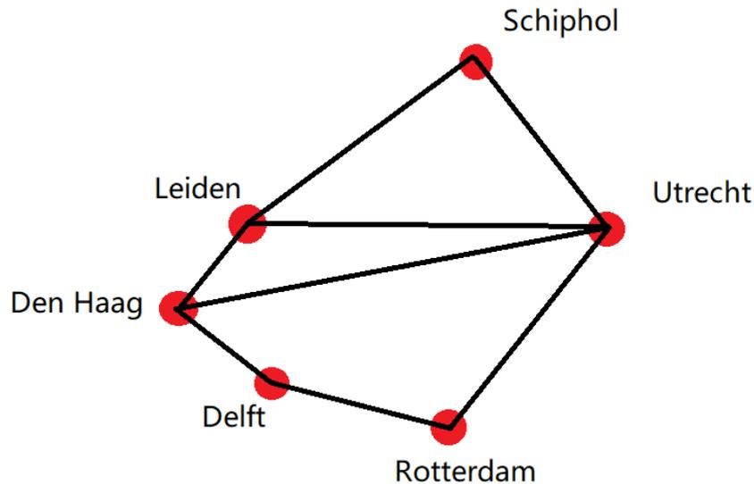
Figure 1.2: A train graph  $G$  with stations as vertices and train tracks as edges. Train connections from [9].
