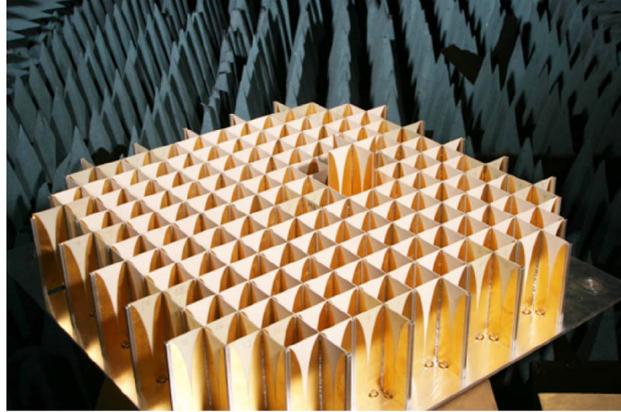
Figure 1.1: A 324-element Vivaldi antenna array [3].
