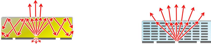
Figure 1.4: Illustration of the enhancement of the front-to-back ratio using (a) homogeneous dielectrics and (b) an artificial dielectric superstrate.
