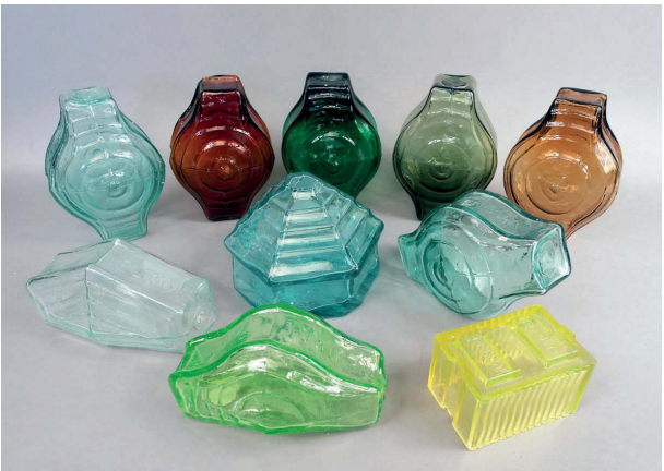
Figure 03.4: Hollow glass blocks (Falconnier. G, 1886)
