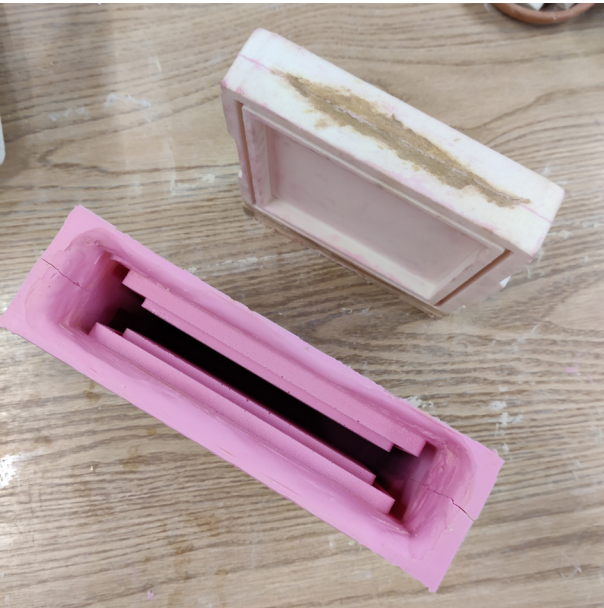
Figure 10.6: Silicone Mold & foam block separated
