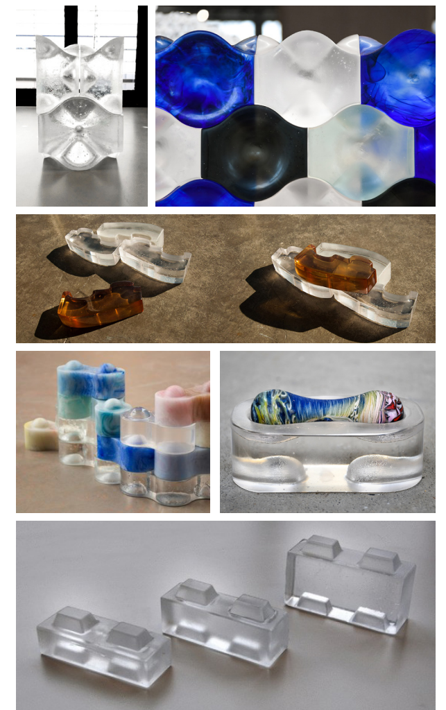
Figure 03.9: Interlocking cast glass geometries ( Oikonomopoulou, F. 2019 )
