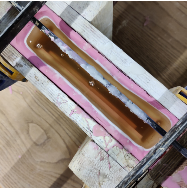
Figure 10.7: Wax pouring inside the silicone mold
