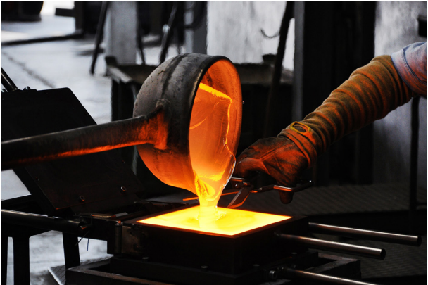
Figure 02.13 : Casting of Soda-lime glass blocks at Poesia factory in Italy (Oikonomopoulou, F, 2019)
