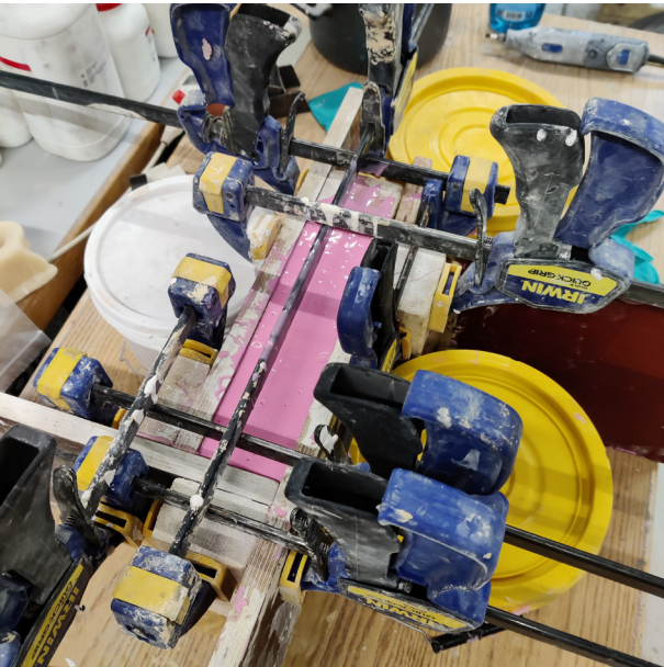
Figure 10.5: Silicone poured inside the bounding box
