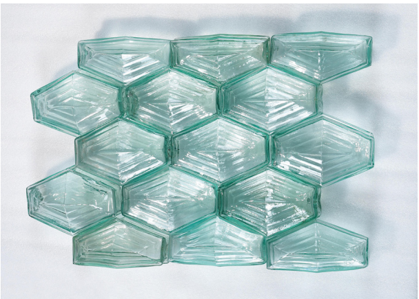
Figure 03.5: Hollow glass blocks (Falconnier. G, 1886)
