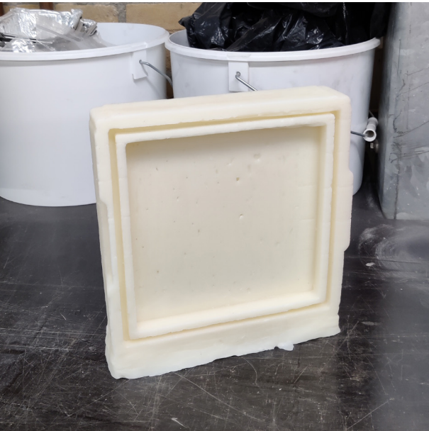
Figure 10.8: Wax block obtained after casting
