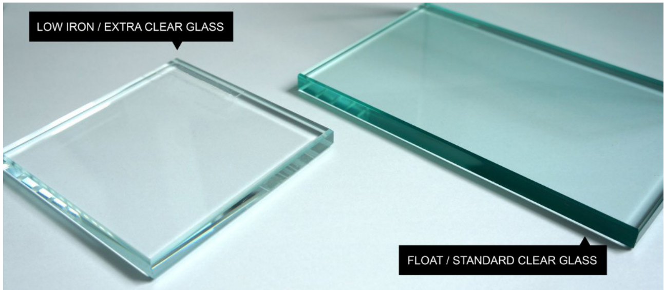
Figure 02.3: Change in glass colour due to the presence of metal oxides retrieved from (Diamond glass)
