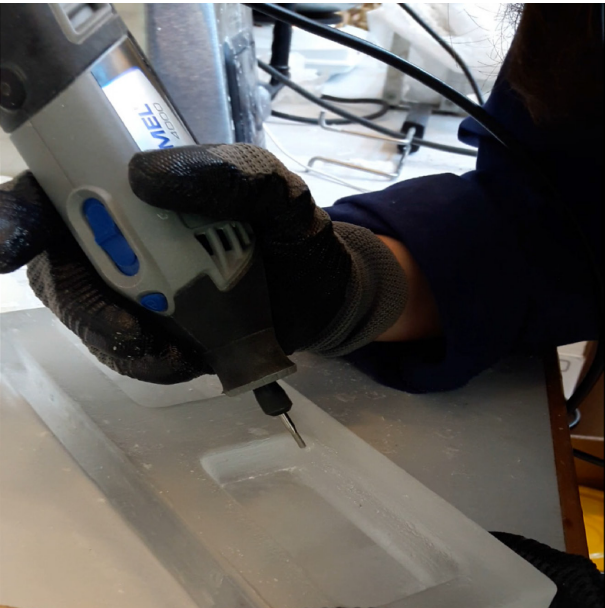
Figure 10.16: Post-processing glass block (Barou. L. 2016)
