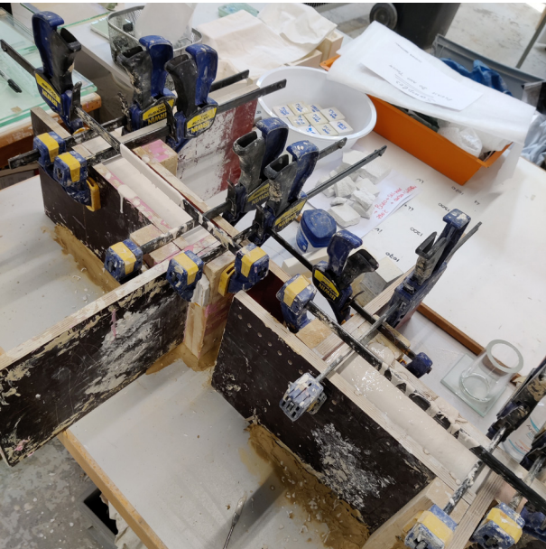
Figure 10.9: Crystal cast poured over the wax block
