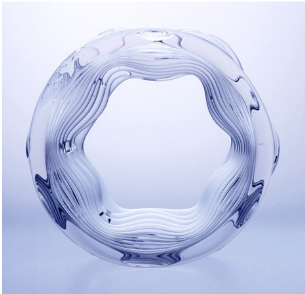
Figure 02.12 : 3D Printed glass component (John Klein)
