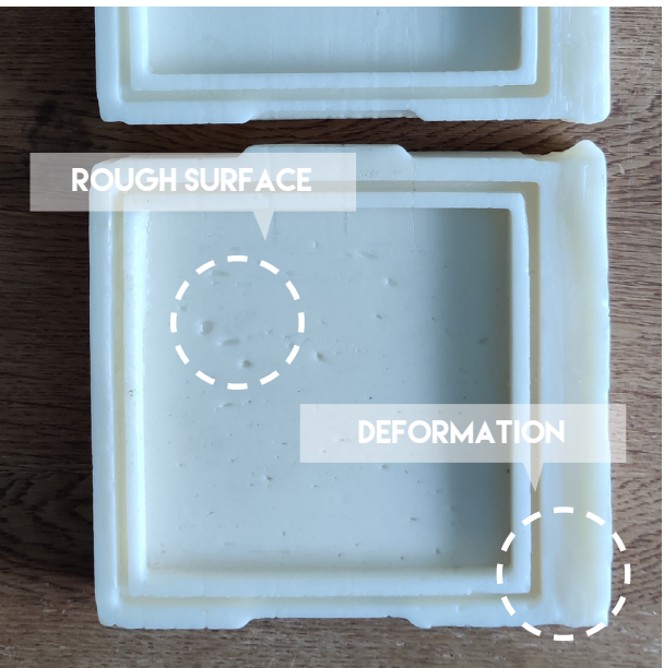
Figure 10.20: Visible deformation and rough surface of the casted wax block.
