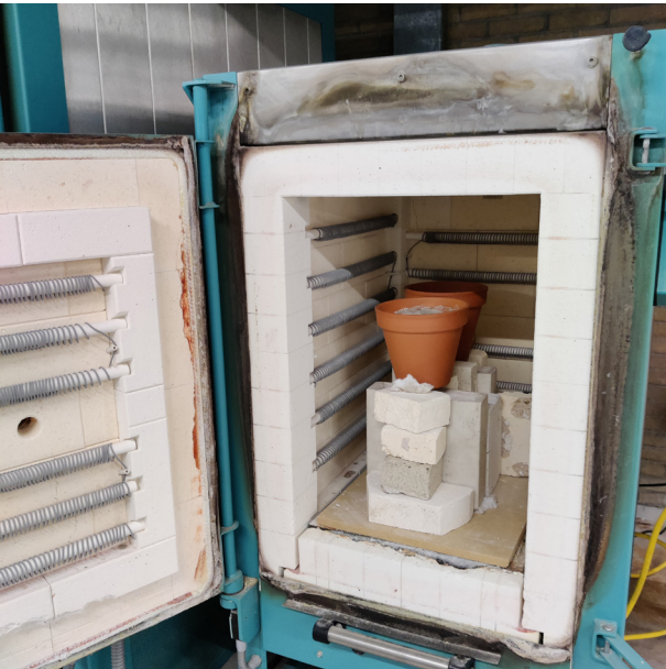
Figure 10.13: Mold set-up inside the kiln for glass casting
