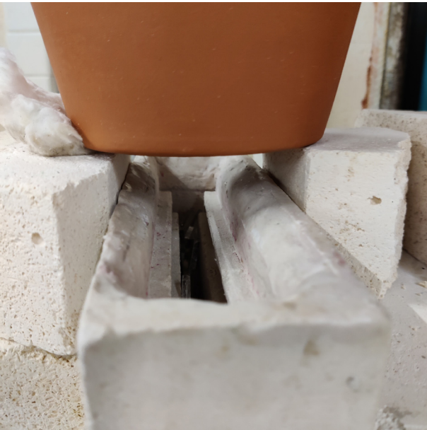
Figure 10.14: Alignment of clay pot opening with the mold
