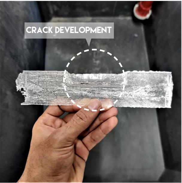
Figure 10.21: Visible cracks at the alignment detail
