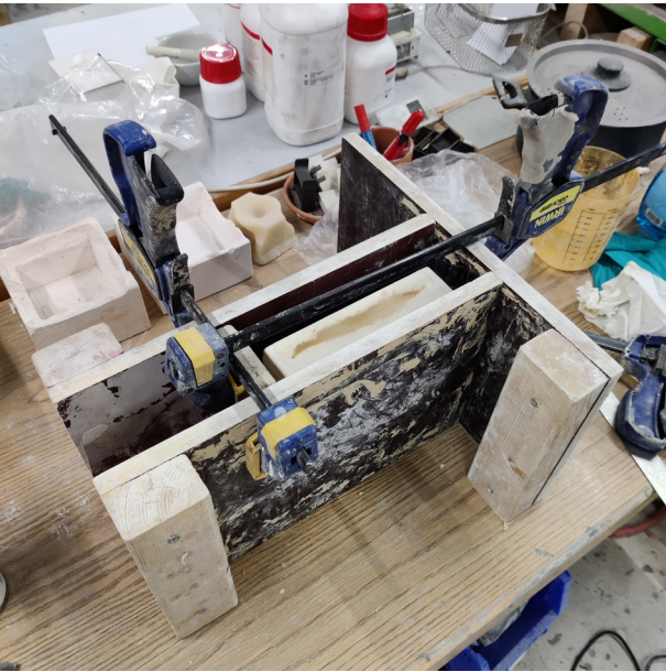
Figure 10.4: Bounding box set-up for the silicone pouring
