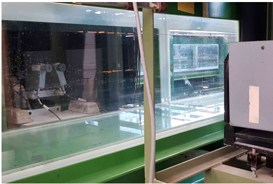
Figure 3.7: LDA emitter and receivers
