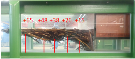
Figure 6.2: Velocity profile measurement locations for conditions of F_0 = 0.25 and h_0/\delta = 1.4 . Values indicate the distance in cm upstream of the inlet.
