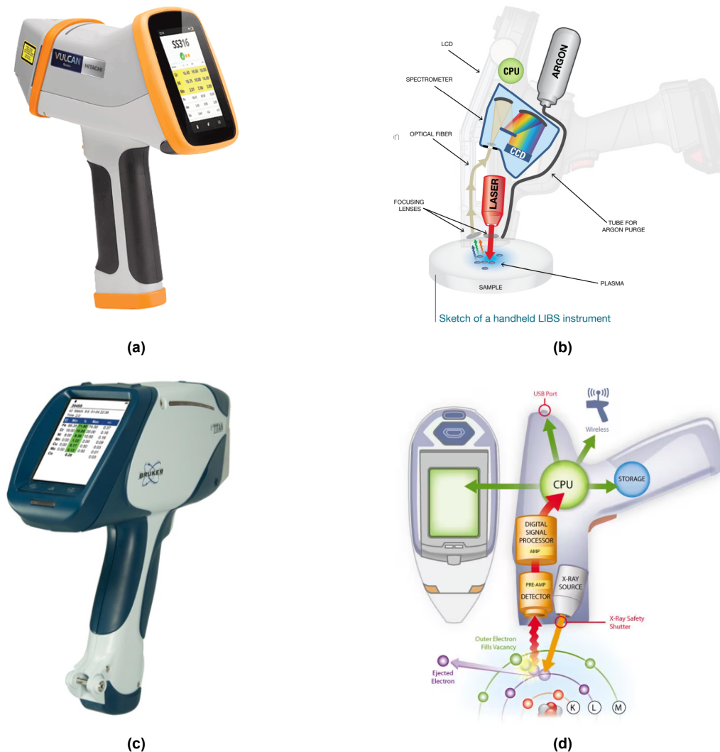
Figure 2.11: Portable non-destructive techniques for analyzing material's composition (a) hLIBS [52]; (b) hLIBS parts and working principle [53]; (c) hXRF [54]; (d) hXRF parts and working principle [55]
