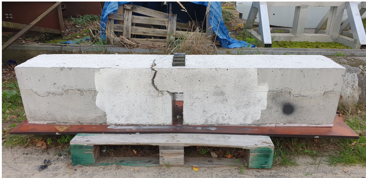
Figure 5.20: Hybrid SHCC-Concrete beam
