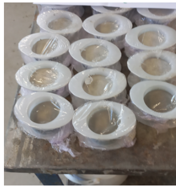
Figure 3.1: Casting cement paste disks
