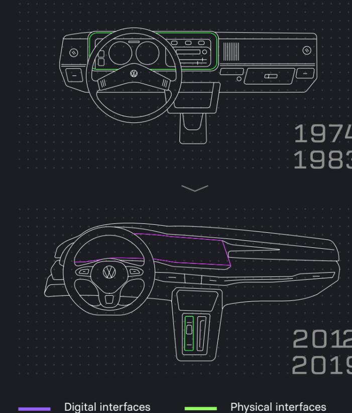
In comparison of both location and type of interface being used in the earliest and latest model VW Golf, it is clear that a shift all the way from a clustered physical interface to a fully virtual interface with almost all functionalities embedded ,aside from the primary driving controls and stalks behind the steering wheel.
