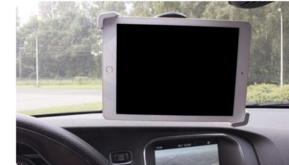
Figure 2a - Tablet obstructing driver's vision
