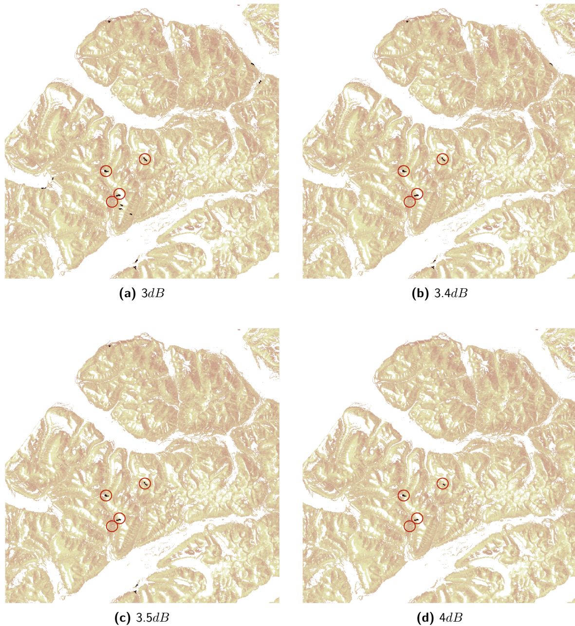
Figure 7.8: Results of automatic detection method using post-classification filter 2: RSO filter and threshold values 3dB , 3.4dB , 3.5dB and 4dB . The method is applied on ascending Sentinel-1A EW difference image from '20150318' and '20150306' in 'HV'-polarisation. Manually detected debris fields are encircled in red. The black areas outside the blue and red circles are false alarms. Increasing the threshold value leads to less false alarms, but also a decrease of probability of detection, i.e. the number of black areas decreases both inside and outside of red circles.
