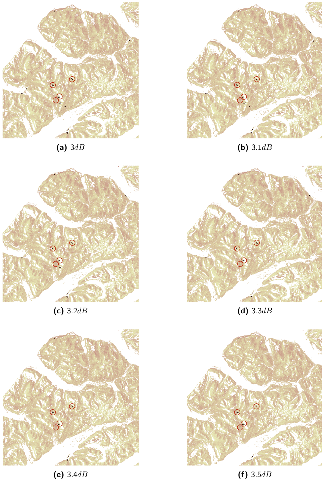
Figure B.8: Results of automatic detection method using post-classification filter 2: RSO filter and threshold values between 3dB and 3.5dB with steps of 0.1dB applied on ascending Sentinel-1A EW difference image from '20150318' and '20150306' in 'HV'-polarisation.
