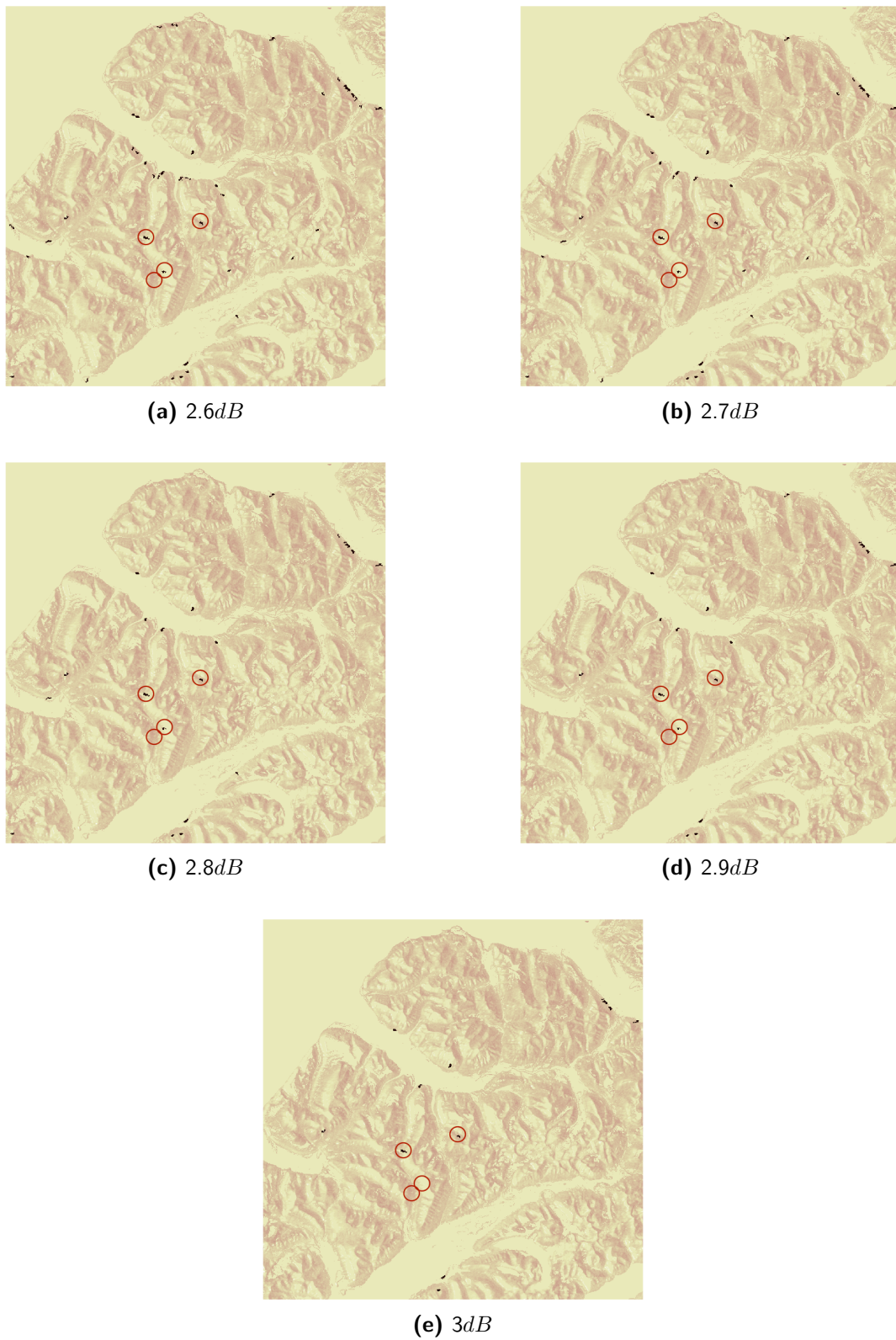
Figure B.11: Results of automatic detection method using post-classification filter 2: RSO filter and threshold values between 2.6dB and 3dB with steps of 0.1dB applied on ascending Sentinel-1A EW difference image from '20150318' and '20150306' in 'HH'-polarisation.
