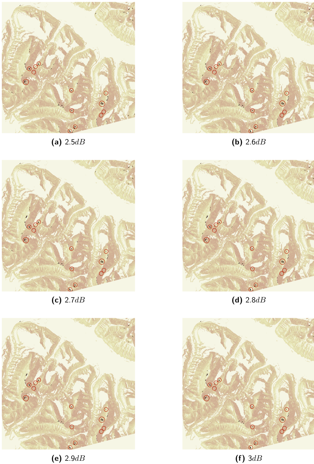
Figure A.9: Results of automatic detection method using post-classification filter 2: RSO filter and threshold values between 2.5dB and 3dB with steps of 0.1dB applied on the ascending RADARSAT-2 UF difference image from '20130610' and '20130914' in 'VV'-polarisation.
