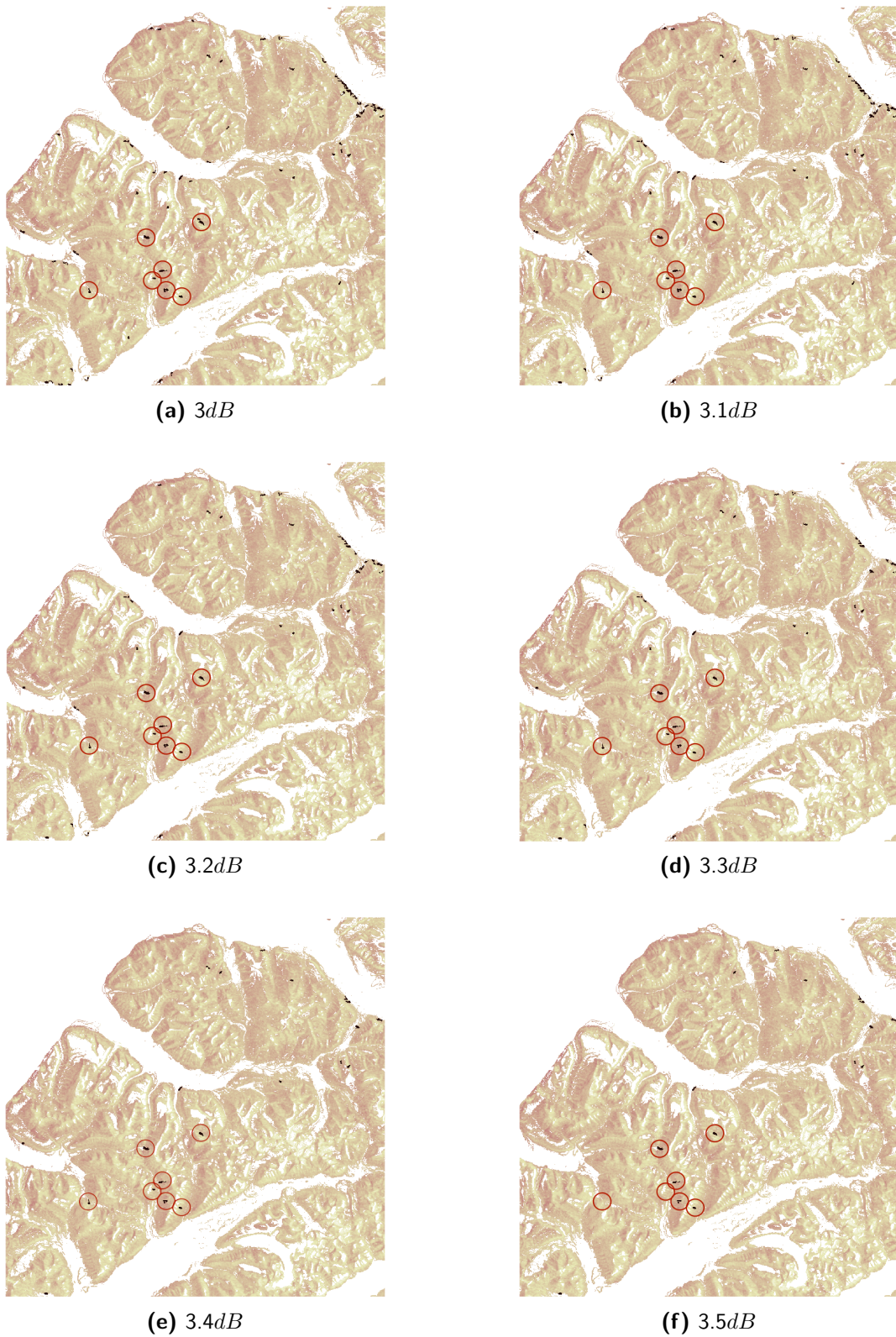
Figure B.4: Results of automatic detection method using post-classification filter 2: RSO filter and threshold values between 3dB and 3.5dB with steps of 0.1dB applied on descending Sentinel-1A EW difference image from '20150318' and '20150306' in 'HV'-polarisation.
