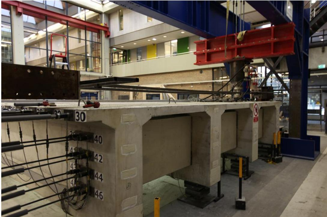
Figure 101 Apparatus of bridge model
