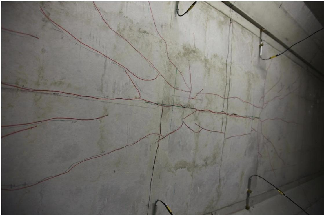
Figure 120 Bottom side of deck slab after failure
