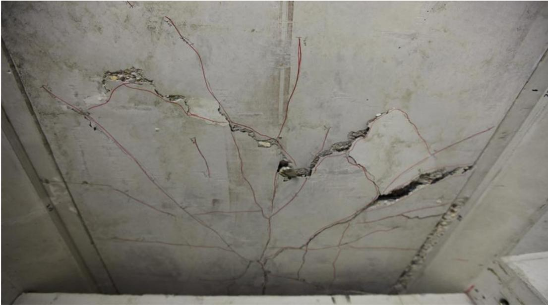
*Figure 105 Bottom side of deck slab after failure*
