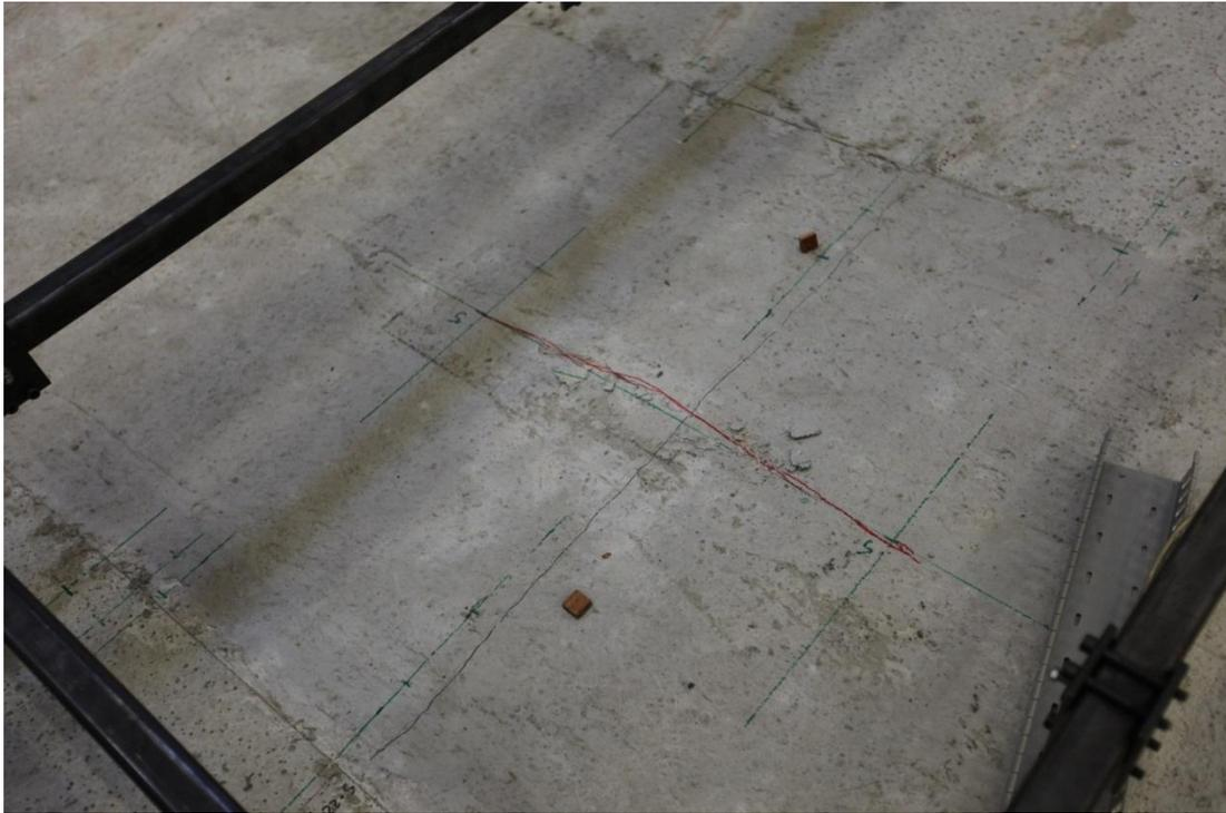
*Figure 121 Top side of deck slab after failure*
