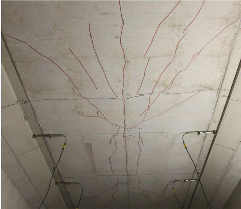
*Figure 124 Bottom side of deck slab after failure*
