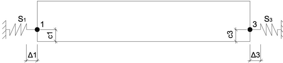
Figure 29 Linear springs at both ends of slab
