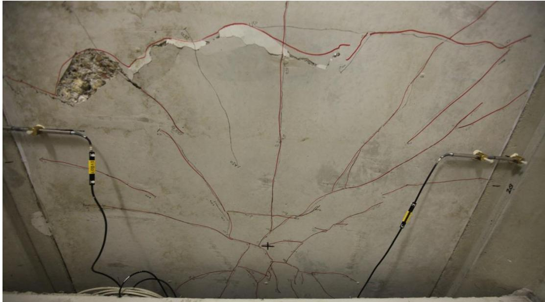
*Figure 111 Bottom side of deck slab after failure*
