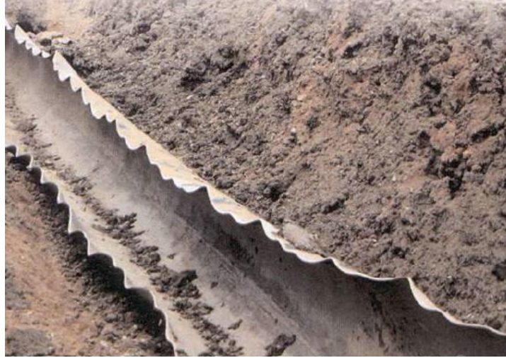
Figure 1.1: Simulation of a pipeline ductile fracture. In the simulation, there is an initial rupture and this gives a snowball effect that propagates the rupture over a large part of the pipeline. Source: Istre [7]
