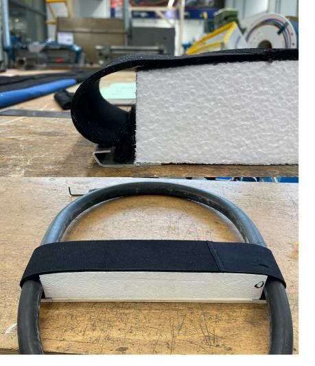
Figure 19 -Prototype of removable shell
