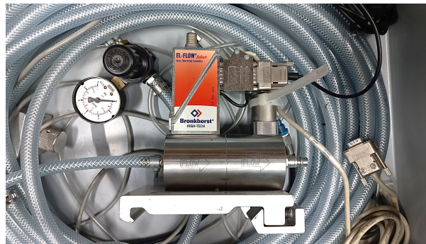
Figure 6.1: Bronkhorst EL-FLOW Select mass-flow controller
