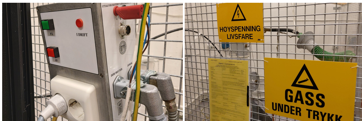
(a) Main switch connected to automatic grounding, HVDC power source, door lock, and live experiment light
