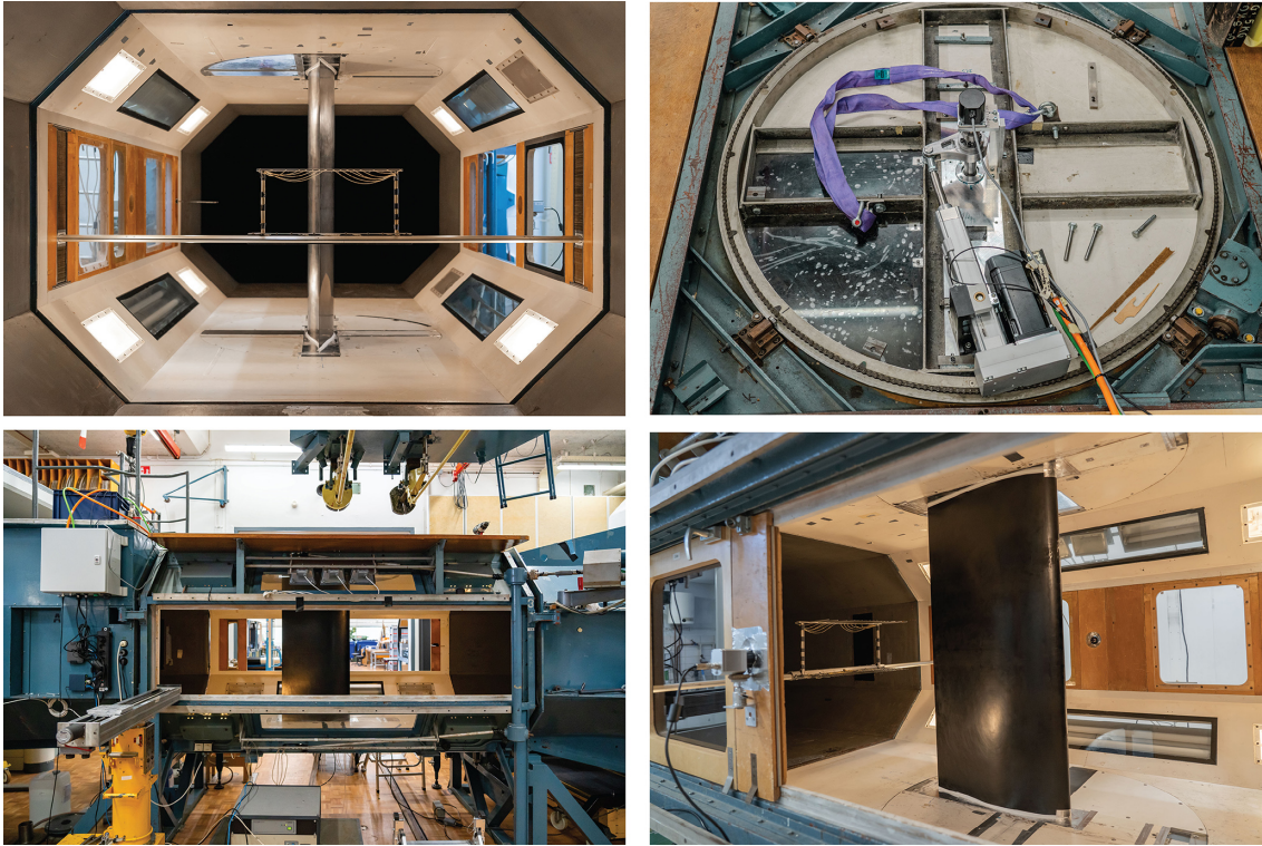
Figure 4. Experimental setup details. The top-left image shows the testing section geometry, with the wake rake behind the airfoil. The linear actuator mechanism is shown in the top-right image. The testing section installed in the wind tunnel is shown in the bottom-left image, without the covering panels for visibility purposes. The airfoil model (with sealed gaps between the wind tunnel walls and airfoil model) is shown in the bottom-right image, with the thermal cameras installed at the airfoil's midspan, for x/c = 50\% .
