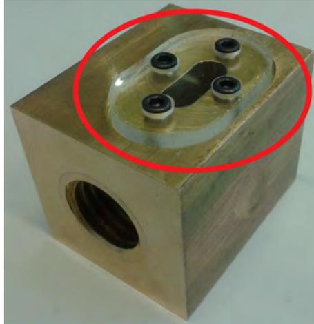
Figure 6.1: Red circle showing the viewing window in the tissue holder
