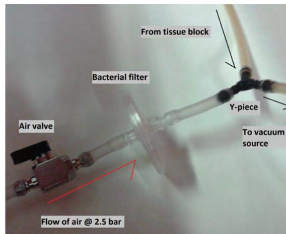
Figure 5.8: Connection of air connection to waste removal
