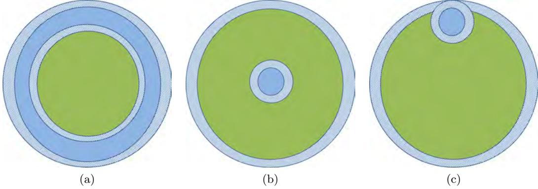
Figure 4.1: The three solutions for the water channel, water ring around suction channel, water channel in the center, and the water channel on the side. Green: waste channel, blue: water channel, striped blue: wall
