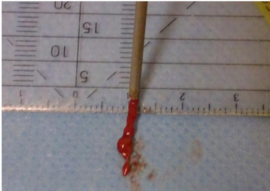
Figure 3.3: Inner diameter 1.1 mm: Waste size 2 mm
