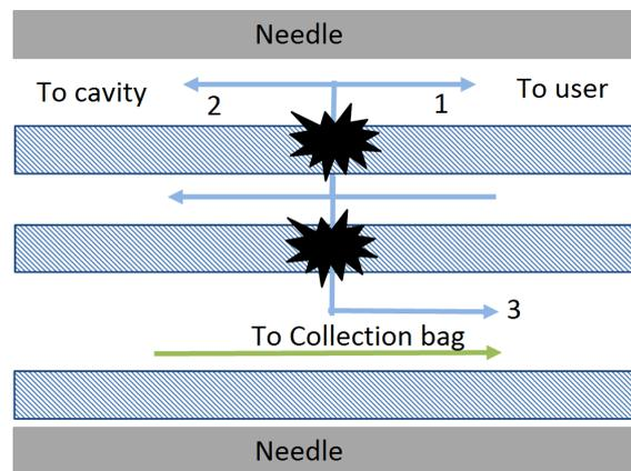
Figure 3.1: Figure schematically showing the three scenarios for a wall which has burst open
