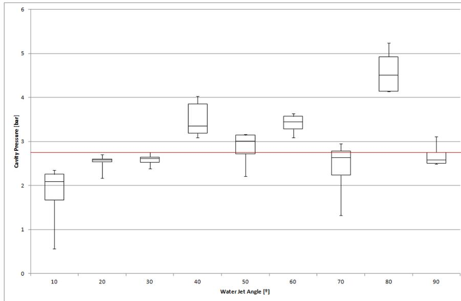
Figure 5.7: Boxplot of peak cavity pressure data for each water jet angle
