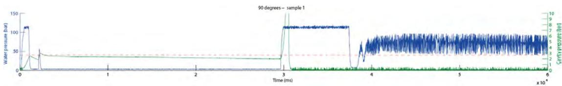
Figure 5.5: Measurement of sample where the relays caused the cavity pressure to rise above 10 bar. Blue: water jet pressure, left y-axis; green: cavity pressure, right y-axis; red dotted line: 2.7 bar threshold, right y-axis
