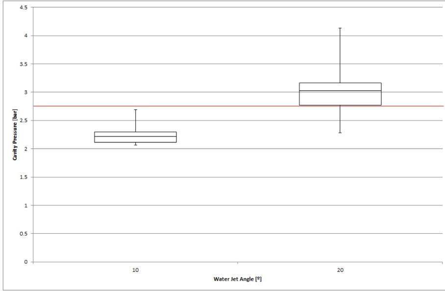
Figure 5.9: Boxplot of the peak cavity pressures for each water jet angle combined with an air pulse
