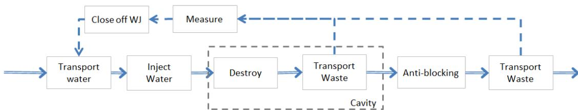
Figure 3.8: Altered functional overview of a water jet dissector from Figure 2.6; solid lines indicate material flow and dashed lines indicate flow of information
