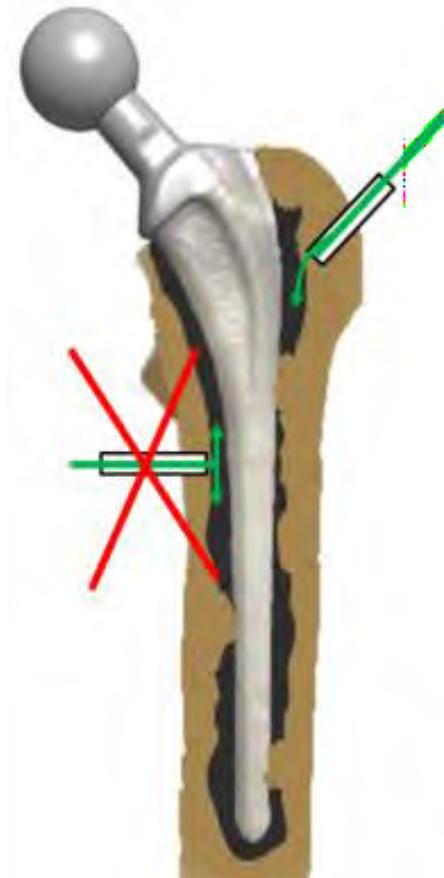
Figure 2.4: Insertion of the instrument, copied from [13], green represents the instrument, black the tissue, and brown the bone.
