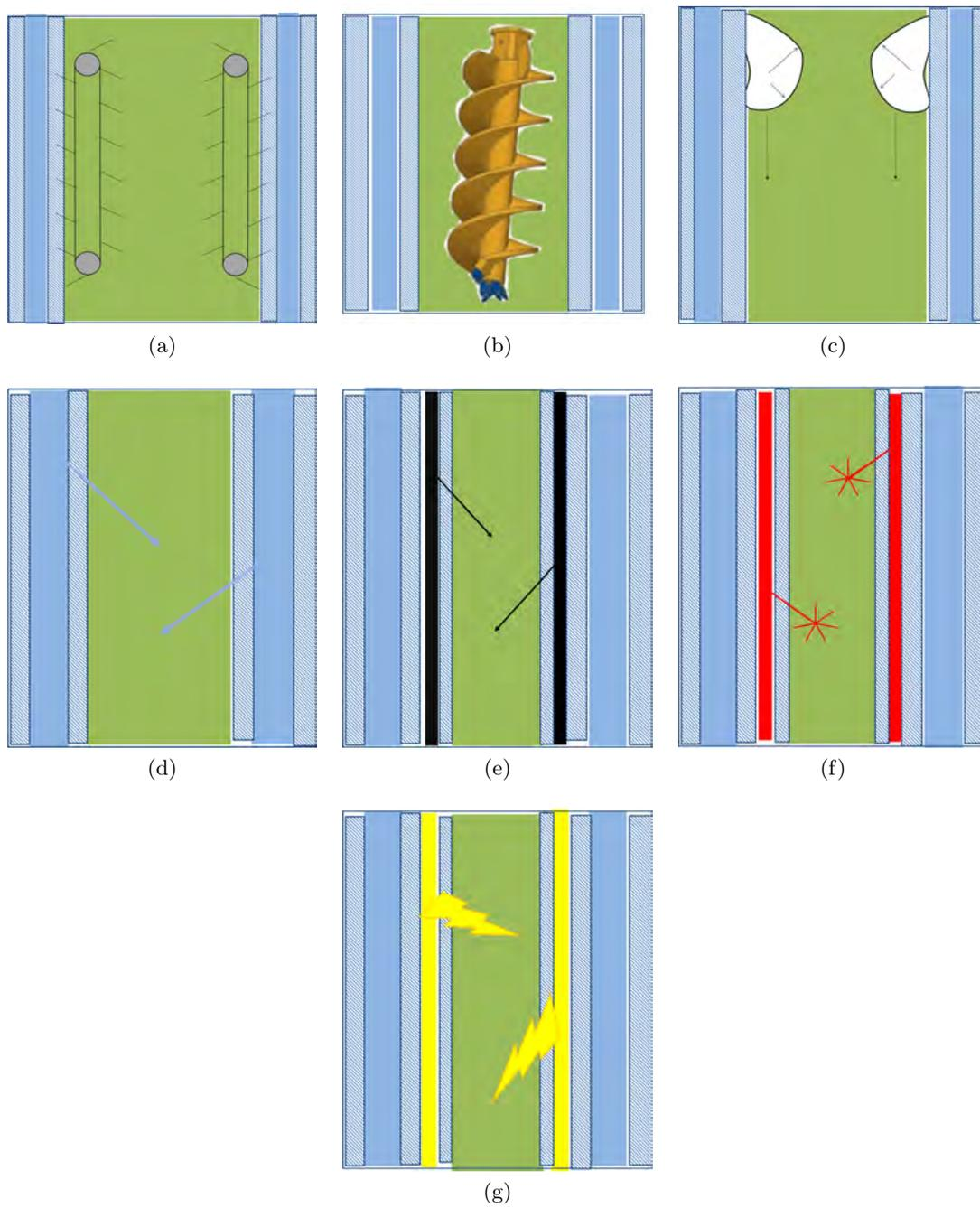
Figure 4.4: Solutions for anti-clogging mechanism
