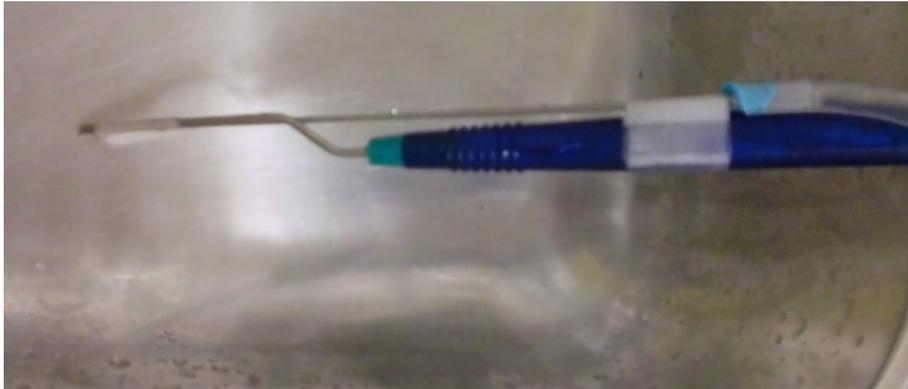
Figure 3.4: Erbe water jet applicator with suction tube connected
