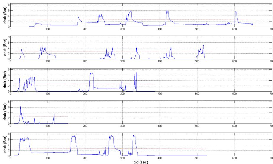
Figure C.1: Graphs showing multiple runs with the Erbe Jet 2 to remove chicken liver whereby the pressure increases above the safety threshold of 2.7 bar
