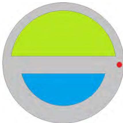
Figure 6.2: Cross-section of instrument (Outer diameter:  $4[mm]$ ): green: waste channel ( $D_{H,suction} = 2.1[mm]$ ), blue: water channel ( $D_{H,WJ} = 1.5[mm]$ ), grey: wall, and red: pressure sensor ( $D = 0.2[mm]$ [29])
