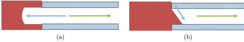
Figure 2.2: The two cases of water jet direction **a** The water jet direction is in line with the instrument. **b** The water jet direction is in counter with the instrument. The green line is the direction in which suction is applied and the blue line is the direction in which the water jet is applied. The blue rectangles with stripes are the walls of the instrument and red resembles tissue.
