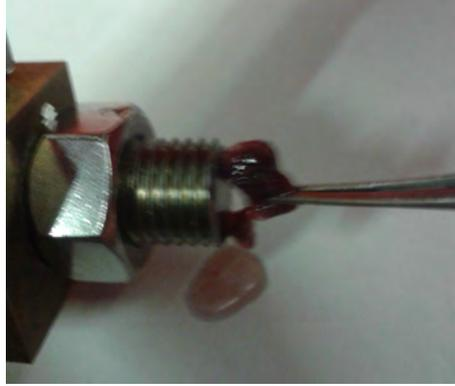
Figure 5.6: Blocked suction tube
