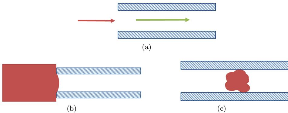
Figure 3.2: **a** Normal situation where there is flow possible as shown by the red and green arrow; **b** Blocked situation, waste blocks the entrance of the suction channel; **c** Clogged situation, waste blocks the inside of the suction channel
