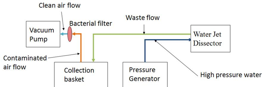
Figure 5.3: Figure schematically showing the experimental setup.
