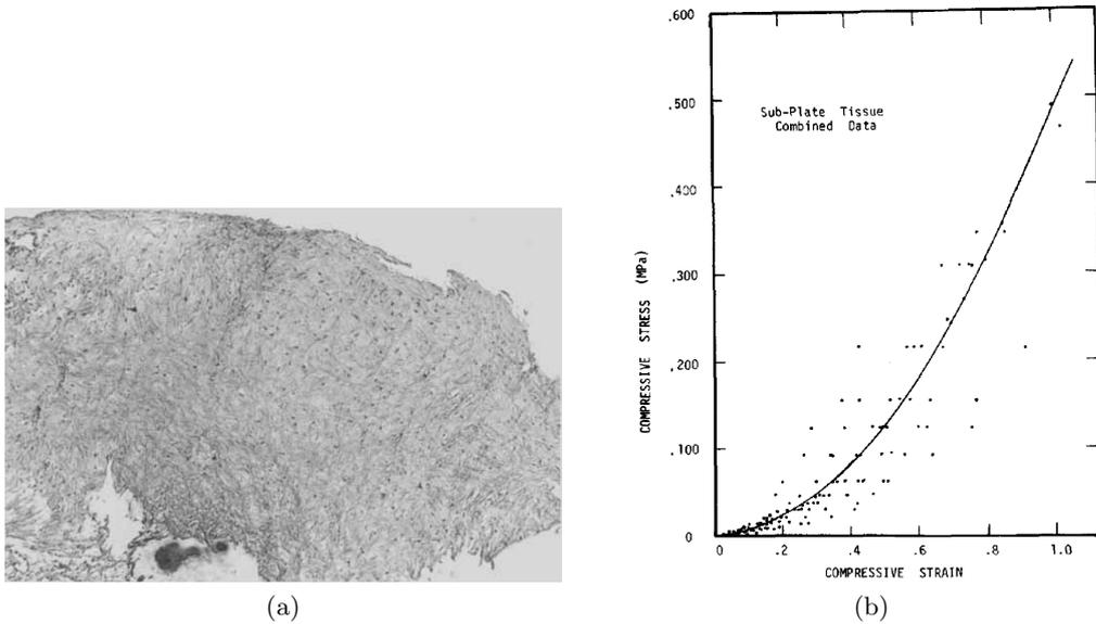
Figure 2.1: **a** Fibrous tissue collected from animal specimen in the study of Hori; **b** Stress-strain curve for unconfined uniaxial compression tests of subplate tissue
