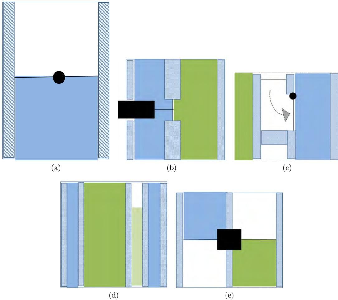
Figure 4.5: Solutions for closing off the water jet channel
