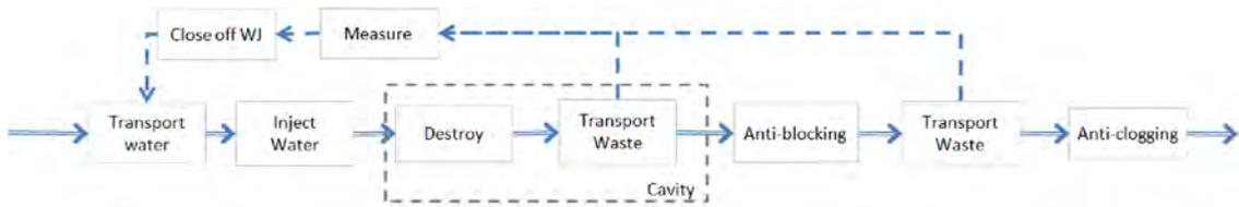
Figure 2.6: Functional overview of a water jet dissector; solid lines indicate material flow and dashed lines indicate flow of information
