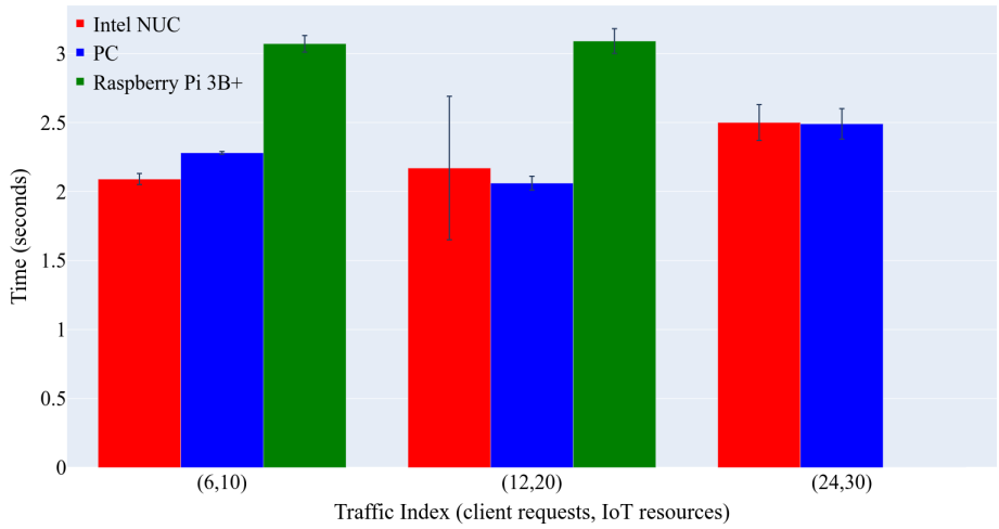
Figure 4.9: Comparison of time taken by EDIRO to serve a client request in bursty traffic scenarios (Raspberry Pi fails to handle a load of 24 concurrent client requests).
