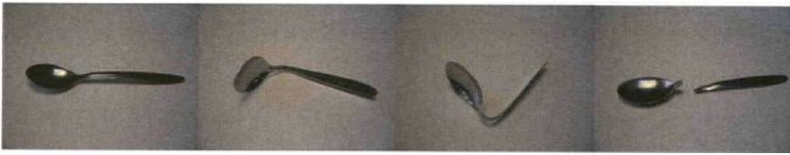
Figure 2.49 Unbent spoon, bending back and forth until breaking
