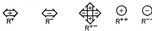
Figure 5.5: Symbols representing the five optimal zones in a beam grid as proposed by Rozvany [95].
