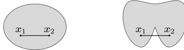
Figure 6.1: Comparison between a convex set (left), and a non-convex or concave set (right) [28].
