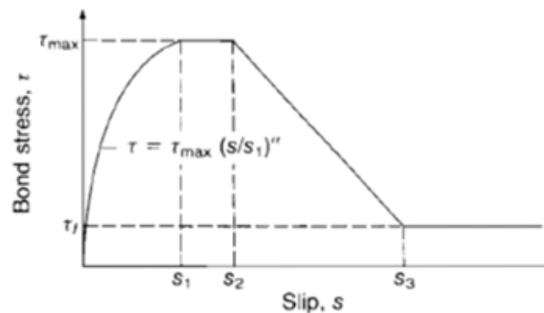
Figure A3 – Parameters used to define bond-slip relation in ATENA (CEB, 1993)
