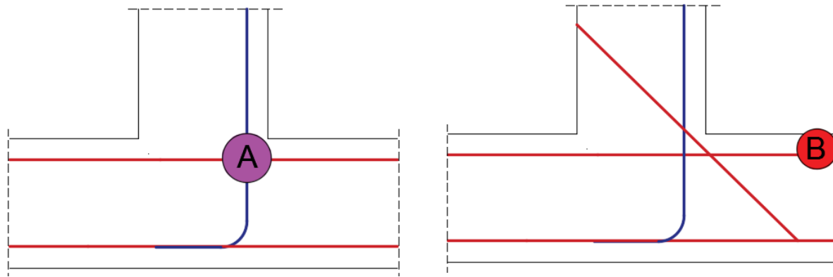
(a) Zone of tensile concentration in variant 5 (b). Zone of tensile concentration in variant 6 Figure 6.12 - Zone of tensile stress concentration and yielding in variants 5 and 6
