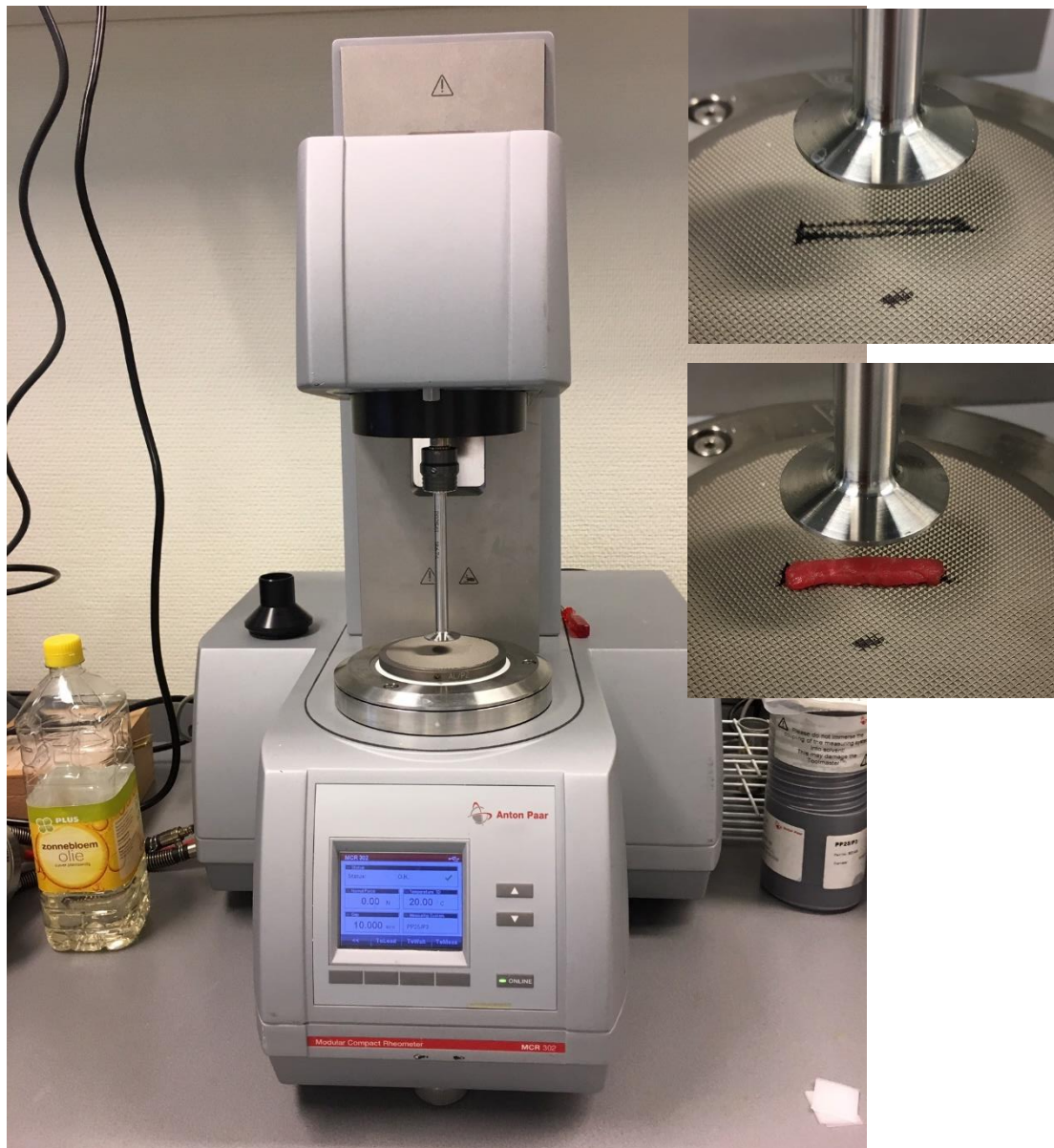
Figure 29. Rheometry measuring device with on the right a zoomed picture of the marked area where samples were placed before testing and a piece of steak placed on this area.
