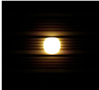
Figure 6.3: **Over-exposure effect.** The white bands in the center of the light blob overlap due to limited exposure settings.
