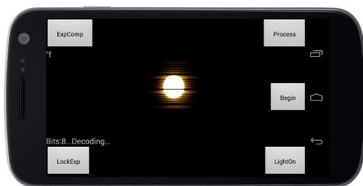
Figure 7.4: **Application screenshot.** The left buttons are used for lowering the exposure time, while the right ones are used for initiating communication and debugging.
