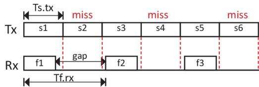
Figure 3.2: **Missing symbols.** If the time gap between the frames is too big there is a high chance of missing symbols or packets.
