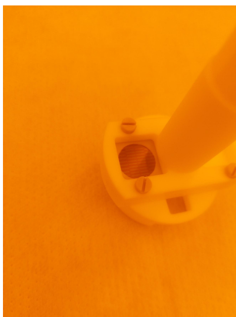
Figure 3.16: The holder used for KOH etching.
