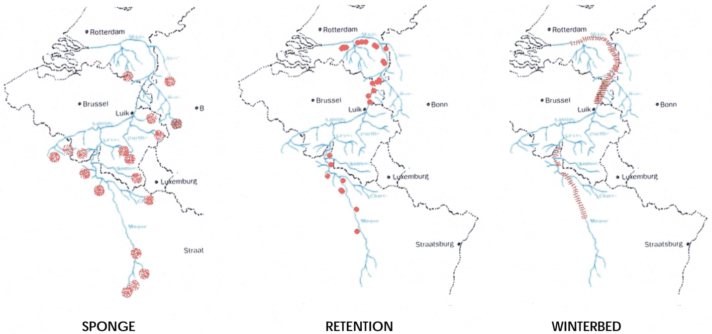
Figure 2.2. Fictive representation of the flood protection strategies used within INTERMEUSE.
