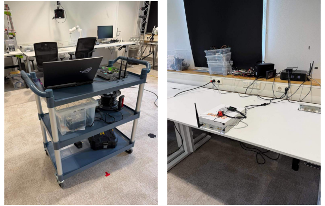
(a) RFSoc receiver setup on the cart. (b) Fixed USRP transmitter setup.
