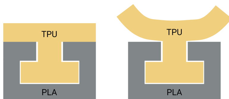
Figure 8.2: Left: TPU and PLA joint using the mechanical interlock when the TPU and PLA are laminated. Right: TPU and PLA joint using mechanical interlock when the TPU and PLA are delaminated during snap-through to the open state of the structure
