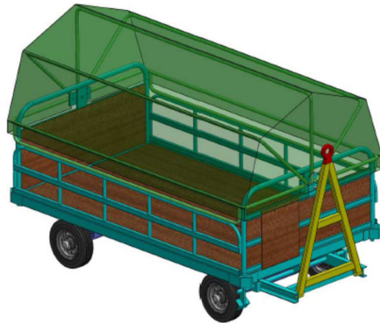
Figure 13: Schematic of a belly/ baggage cart
