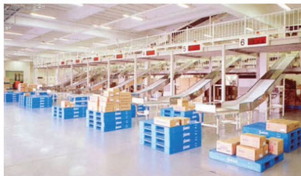
Figure 11: Example of a sorter system
